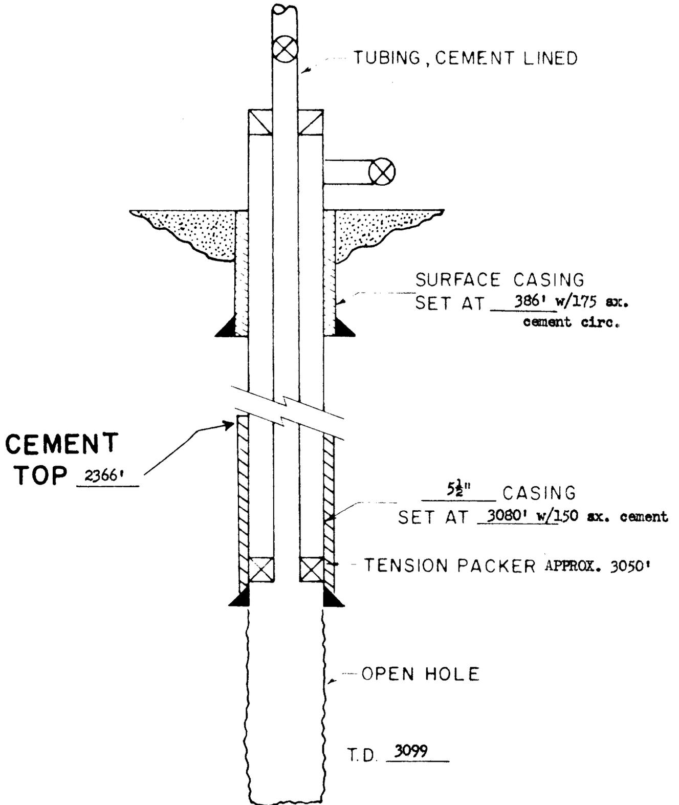
WATER INJECTION WELL SCHEMATIC
