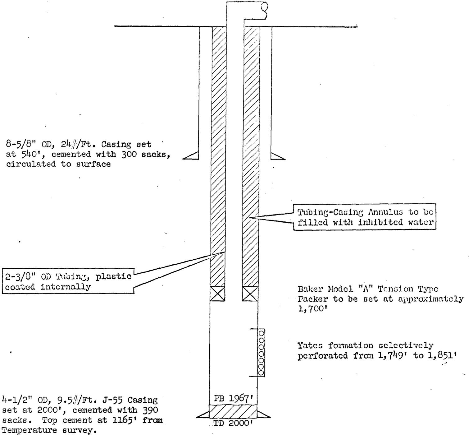
8-5/8" OD, 24#/Ft. Casing set at 540', cemented with 300 sacks, circulated to surface
