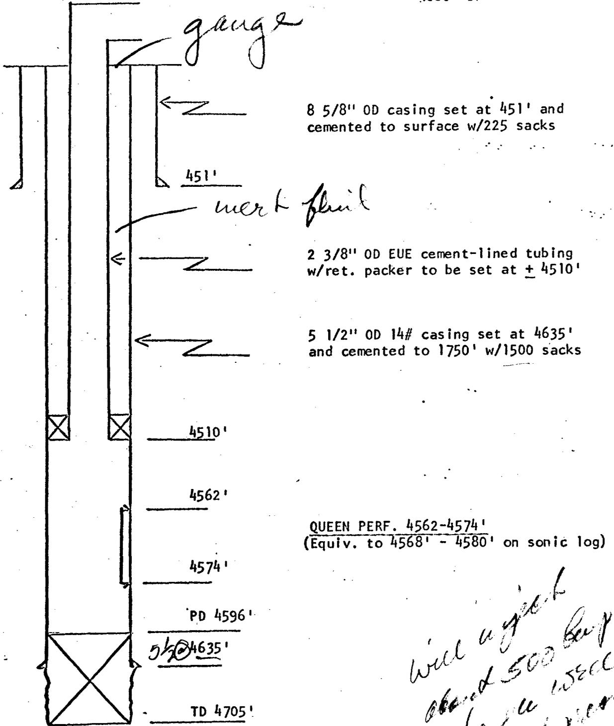
8 5/8" OD casing set at 451' and cemented to surface w/225 sacks
