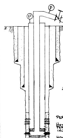
13-36" OD, 48", H-40, STEC SURFACE CASING AT 355'. TO C AT SURFACE (420 5x).
