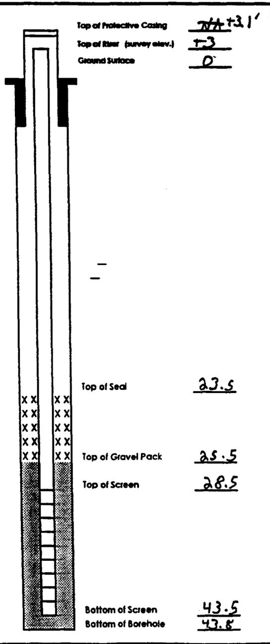
Comment Set well @ 43.5' BGS. Hydrate seal w/ 10 gal potable water. Padlock & locking wellcap on well. Well completed
