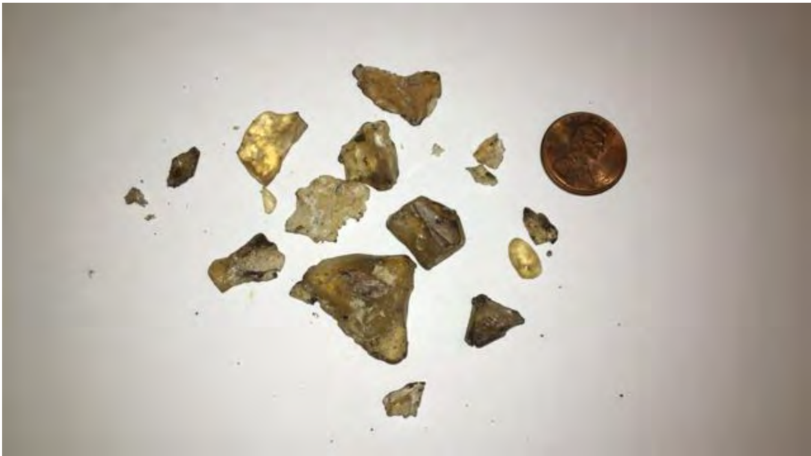
Figure 1 – Resin Cement from Drill Out Operations
