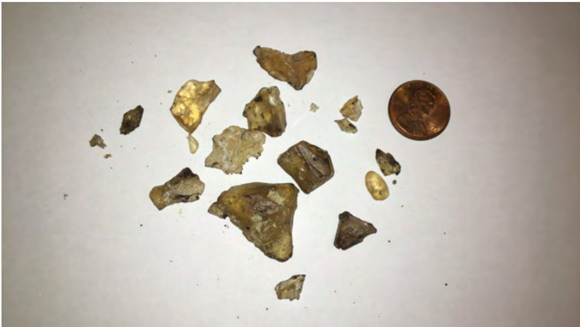
Figure 1 – Resin Cement from Drill Out Operations
