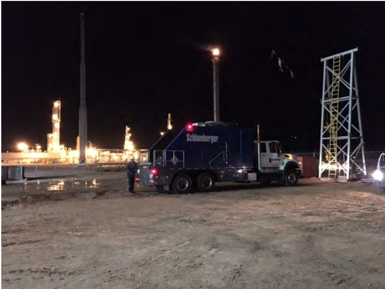
Figure 1 – Open Hole Logging in Injection Zone
