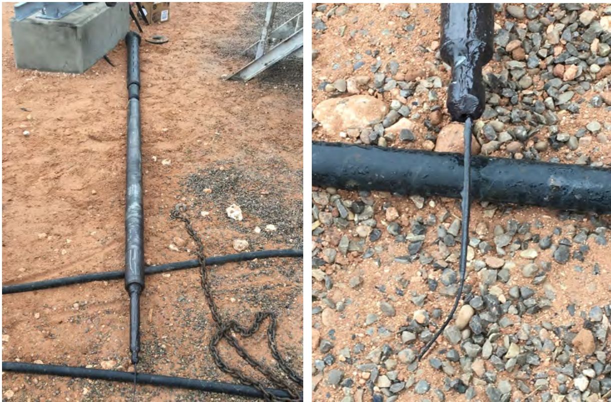
Figure 2 Recovered Halliburton Gauge Ring / CCL Tool
