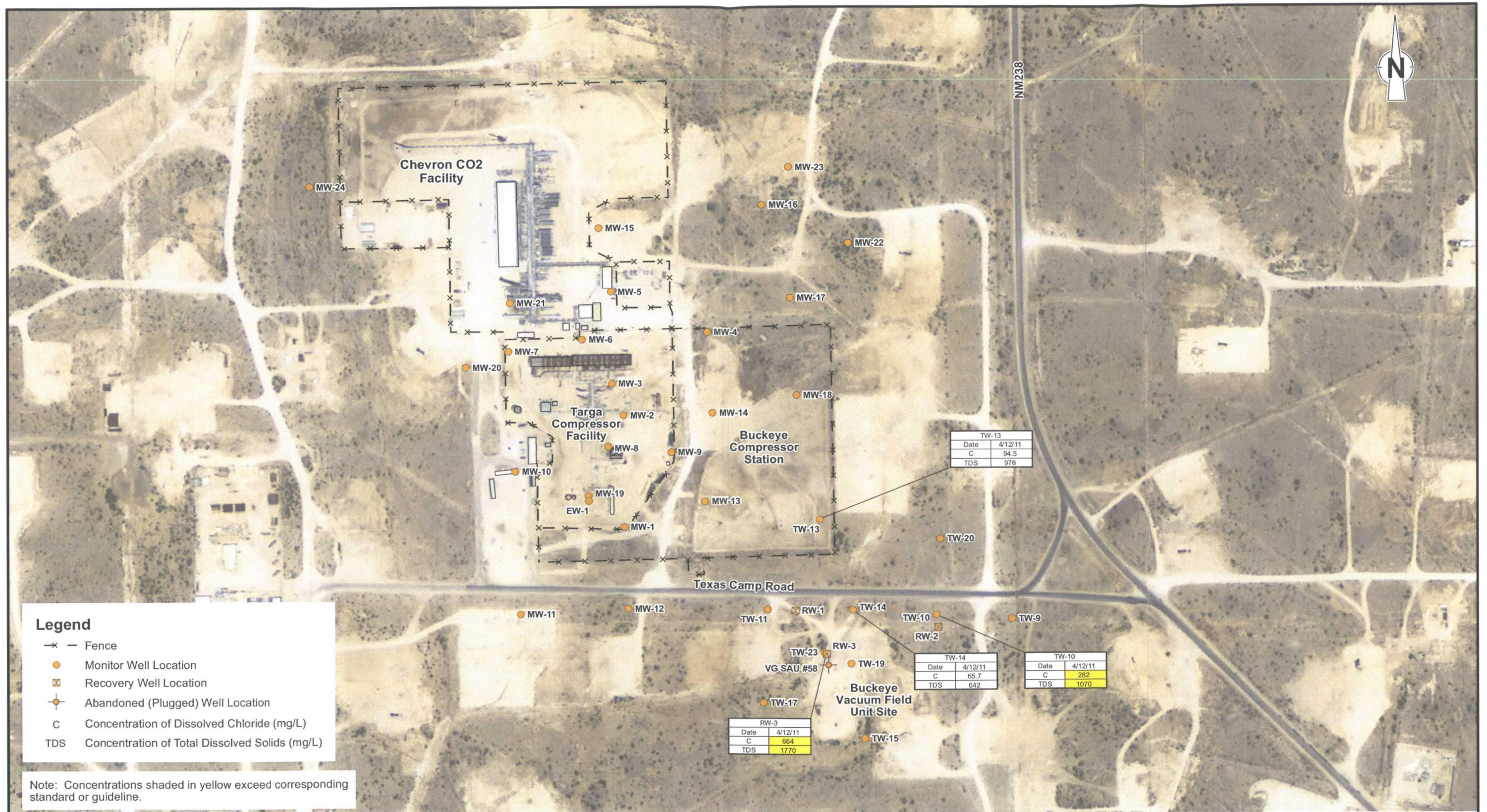
figure 5 DISTRIBUTION OF DISSOLVED CHLORIDE AND TOTAL DISSOLVED SOLIDS - APRIL 12, 2011 BUCKEYE VACUUM FIELD UNIT SITE SECTION 1, T18S-R34E, LEA COUNTY, NEW MEXICO Chevron Environmental Management Company, Houston, Texas
