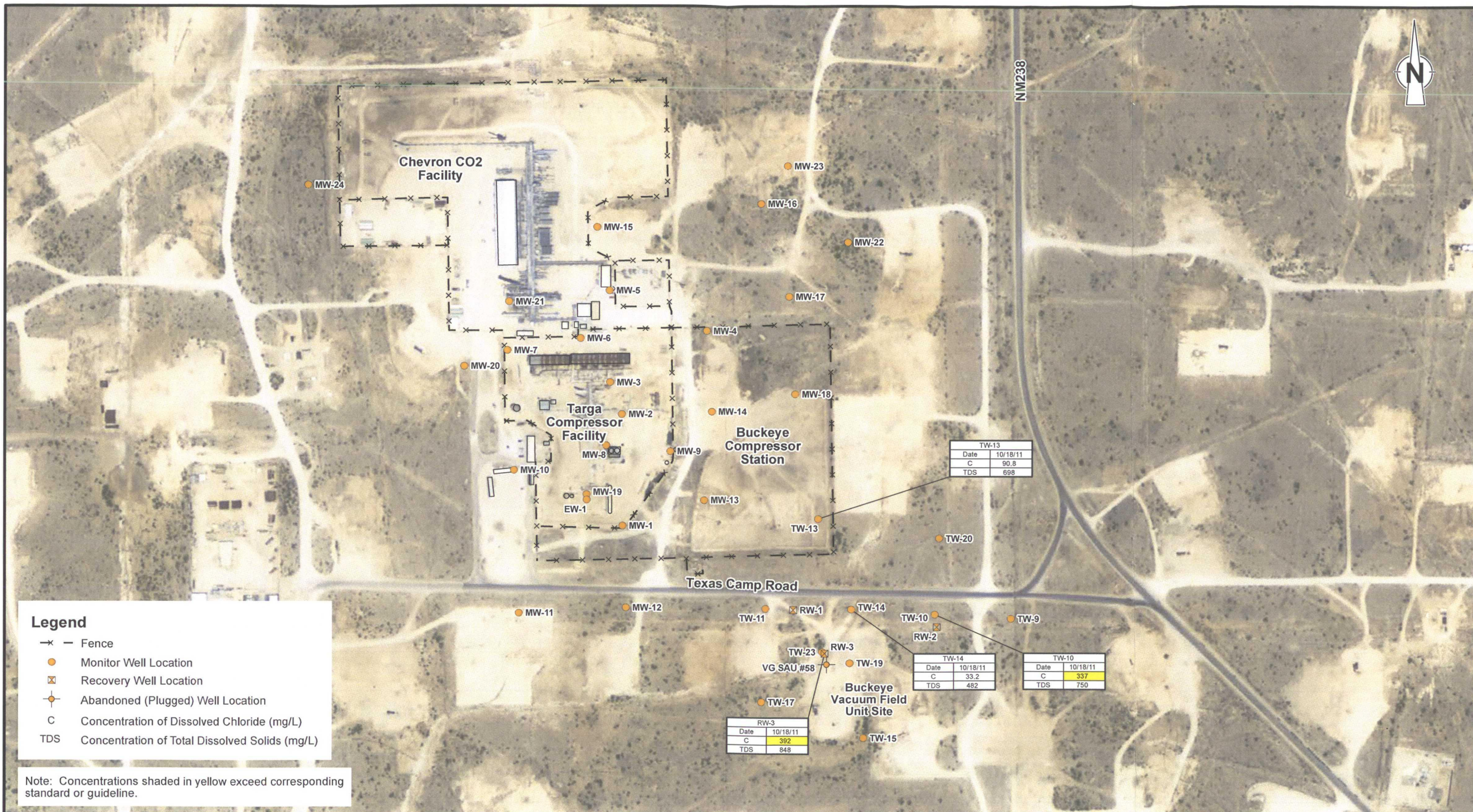
figure 6 DISTRIBUTION OF DISSOLVED CHLORIDE AND TOTAL DISSOLVED SOLIDS - OCTOBER 18, 2011 BUCKEYE VACUUM FIELD UNIT SITE SECTION 1, T18S-R34E, LEA COUNTY, NEW MEXICO Chevron Environmental Management Company, Houston, Texas
