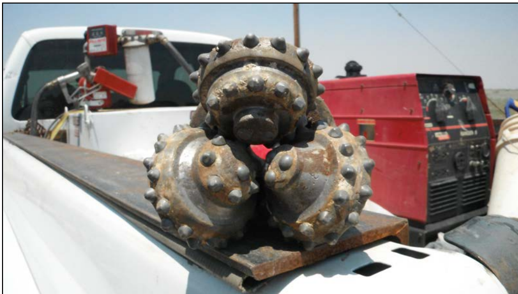
No. 2 – View of the tricone bit used during air rotary drilling.
