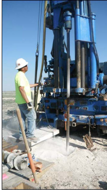
No. 3 – View of air rotary drilling at SB-05.
