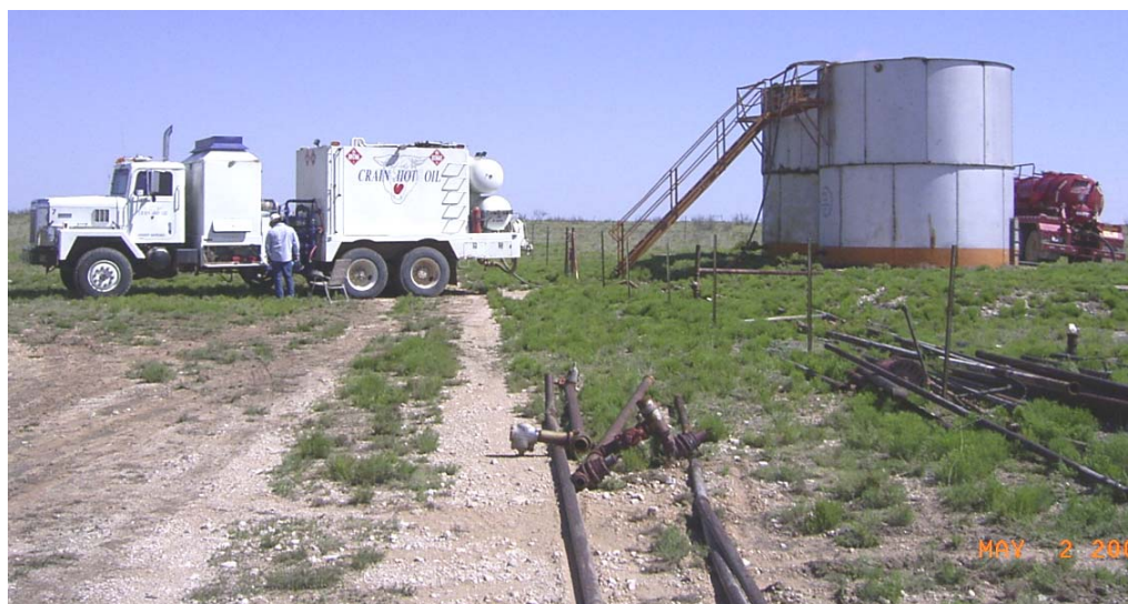
Figure 4. Hot Oil Unit and Two 500-Barrel Bolted Steel Tanks. In the foreground is piping staged for the NORM survey and removal.
