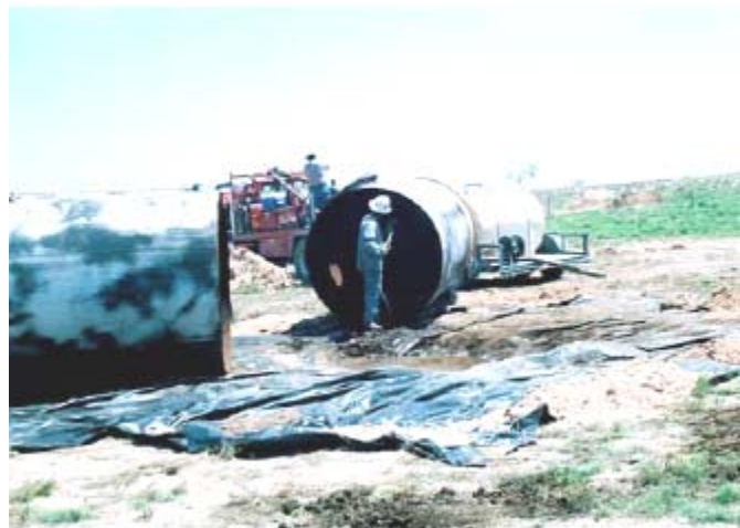
Figure 6. Heater Treater Being Cleaned
