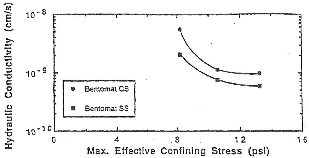
Fig. 2.2 Results of Flexible-Wall Hydraulic Conductivity Tests on Bentomat® (J&L Testing Company, 1990)
