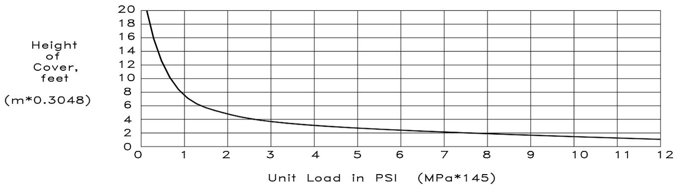
**Note:** The H20 live load assumes two 16,000 lb. loads applied to two 18" x 20" areas, one located over the point in question, and the other located at a distance of 72" away. In this manner, a truckload of 20 tons is simulated.
