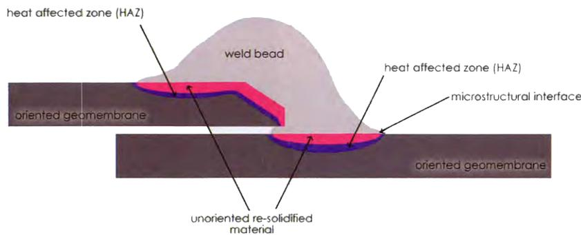
Figure 4 | Schematic of microstructure at extrusion weld
