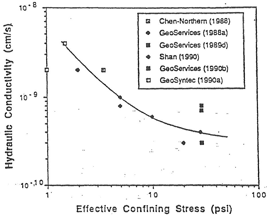
Fig. 2.5 Results of Hydraulic Conductivity Tests on Claymax® Permeated with Water
