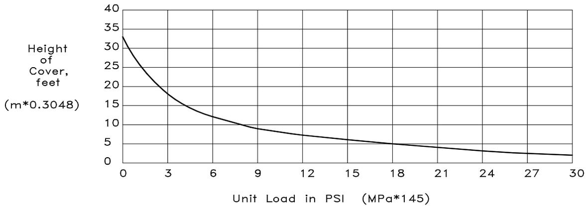
**Note:** The Cooper E-80 live load assumes 80,000 pounds applied to three 2' x 6' areas on 5' centers, such as might be encountered through live loading from a locomotive with three 80,000 pounds axle loads.
