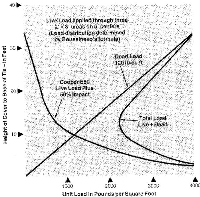
Note: Cooper E-80 live load assumes 80,000 pounds applied to three 2' x 8' areas on 5' centers such as might be encountered through live loading from a locomotive with three 80,000 pound axle loads.
