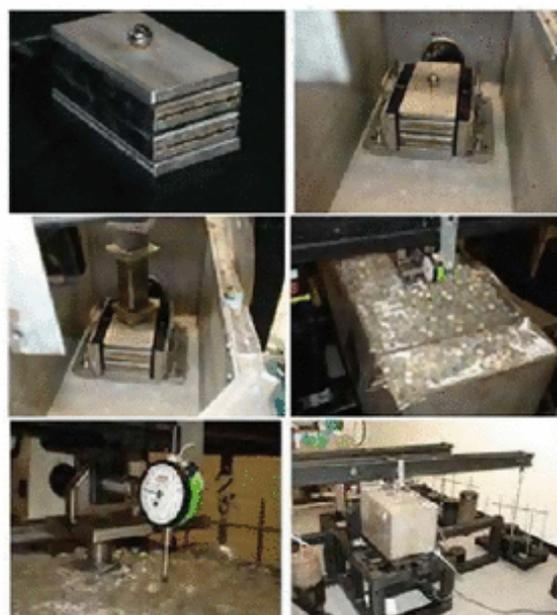
**Fig. 2** Compressive environmental stress cracking test equipment
