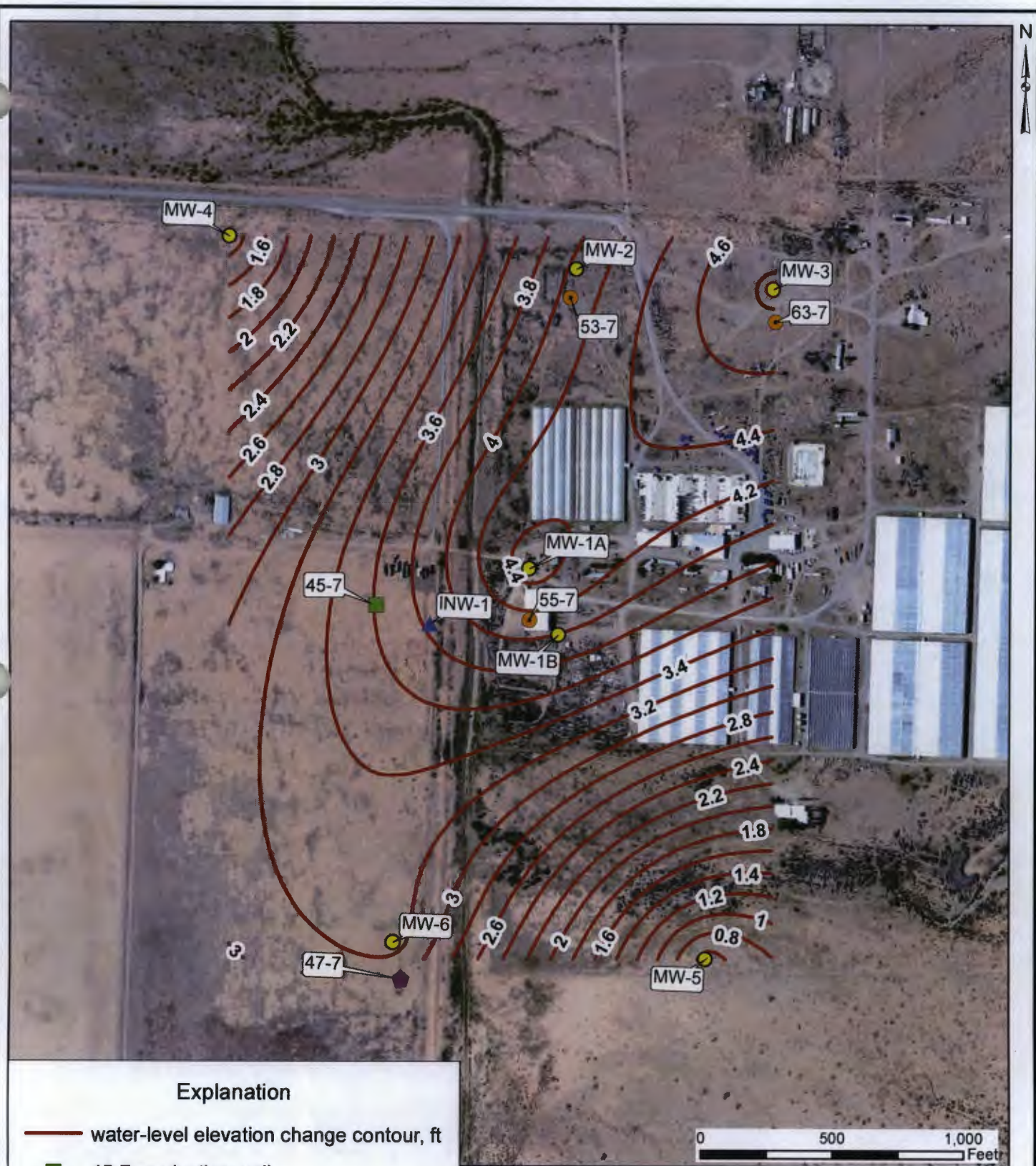
Figure 15. Water-level elevation change in shallow monitoring wells (MW- wells) between December 09, 10, and 11, 2013 (prior to beginning of geothermal operations) and April 17, 2014, Cyrq Energy Lightning Dock Geothermal project. Contour values in feet. Positive value indicates water-level rise.
