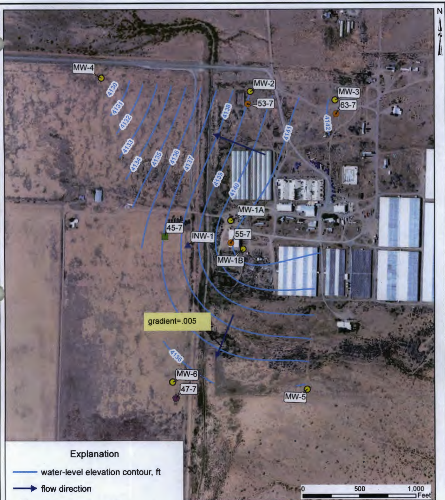
Figure 10. Water-level elevation levels shown in shallow monitoring wells (MW- wells) for May 11, 2014, Cyrq Energy Lightning Dock Geothermal project. Contour values in feet.
