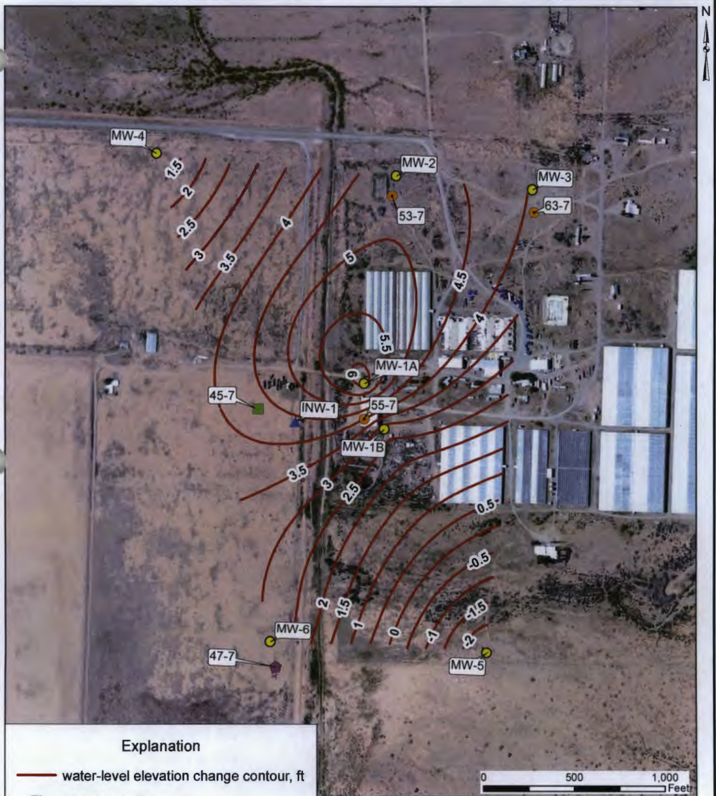
Figure 17. Water-level elevation change in shallow monitoring wells (MW- wells) between December 09, 10, and 11, 2013 (prior to beginning of geothermal operations) and June 19, 2014, Cyrq Energy Lightning Dock Geothermal project. Contour values in feet. Positive value indicates water-level rise.
