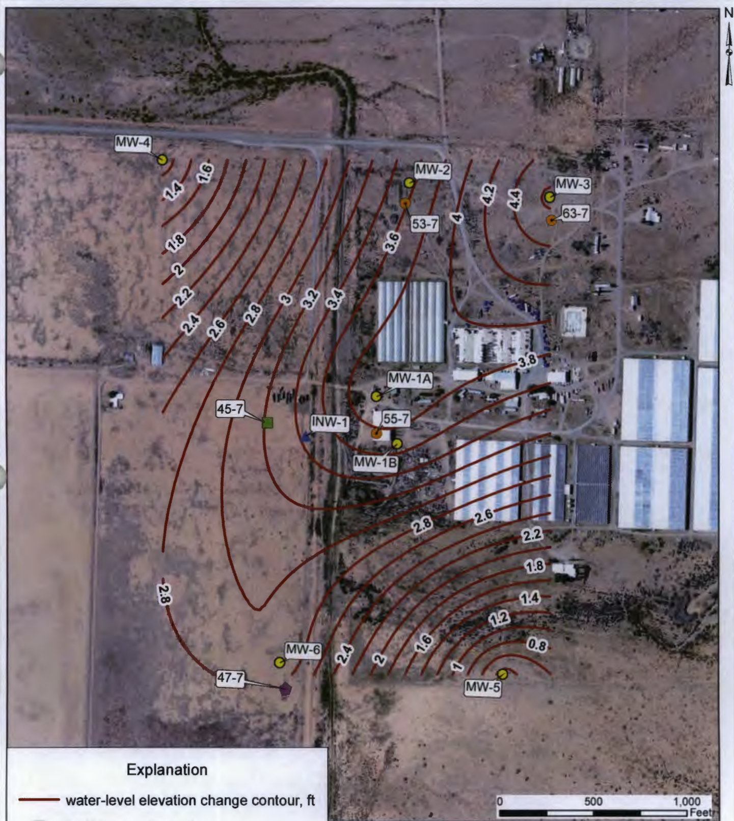
Figure 14. Water-level elevation change in shallow monitoring wells (MW- wells) between December 09, 10, and 11, 2013 (prior to beginning of geothermal operations) and March 17, 2014, Cyrg Energy Lightning Dock Geothermal project. Contour values in feet. Positive value indicates water-level rise.
