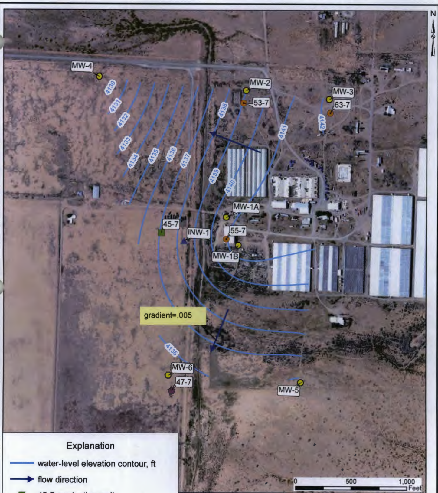
Figure 11. Water-level elevation levels shown in shallow monitoring wells (MW- wells) for June 19, 2014, Cyrq Energy Lightning Dock Geothermal project. Contour values in feet.
