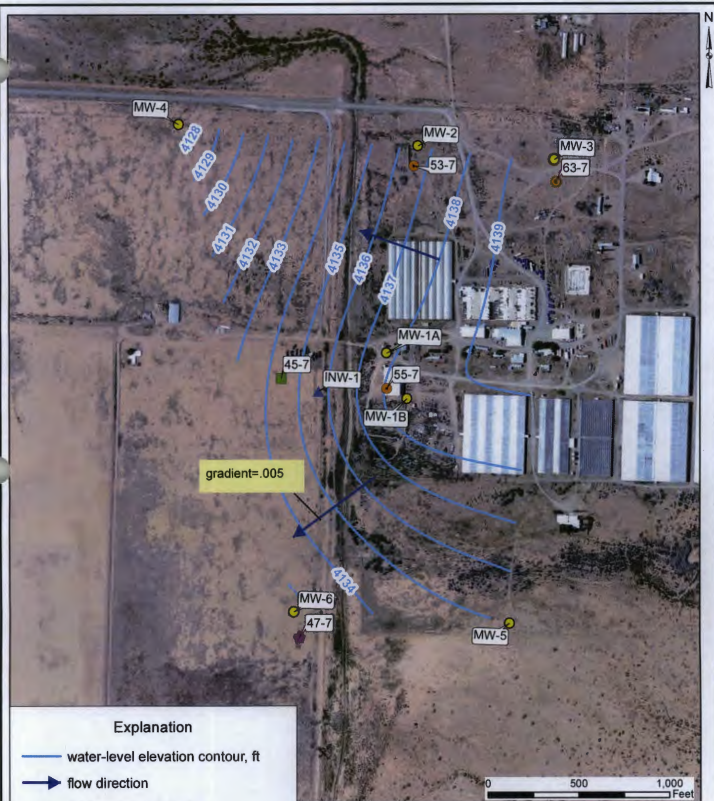
Figure 5. Water-level elevation levels shown in shallow monitoring wells (MW- wells) for December 28, 2013, Cyrq Energy Lightning Dock Geothermal project. Contour values in feet.
