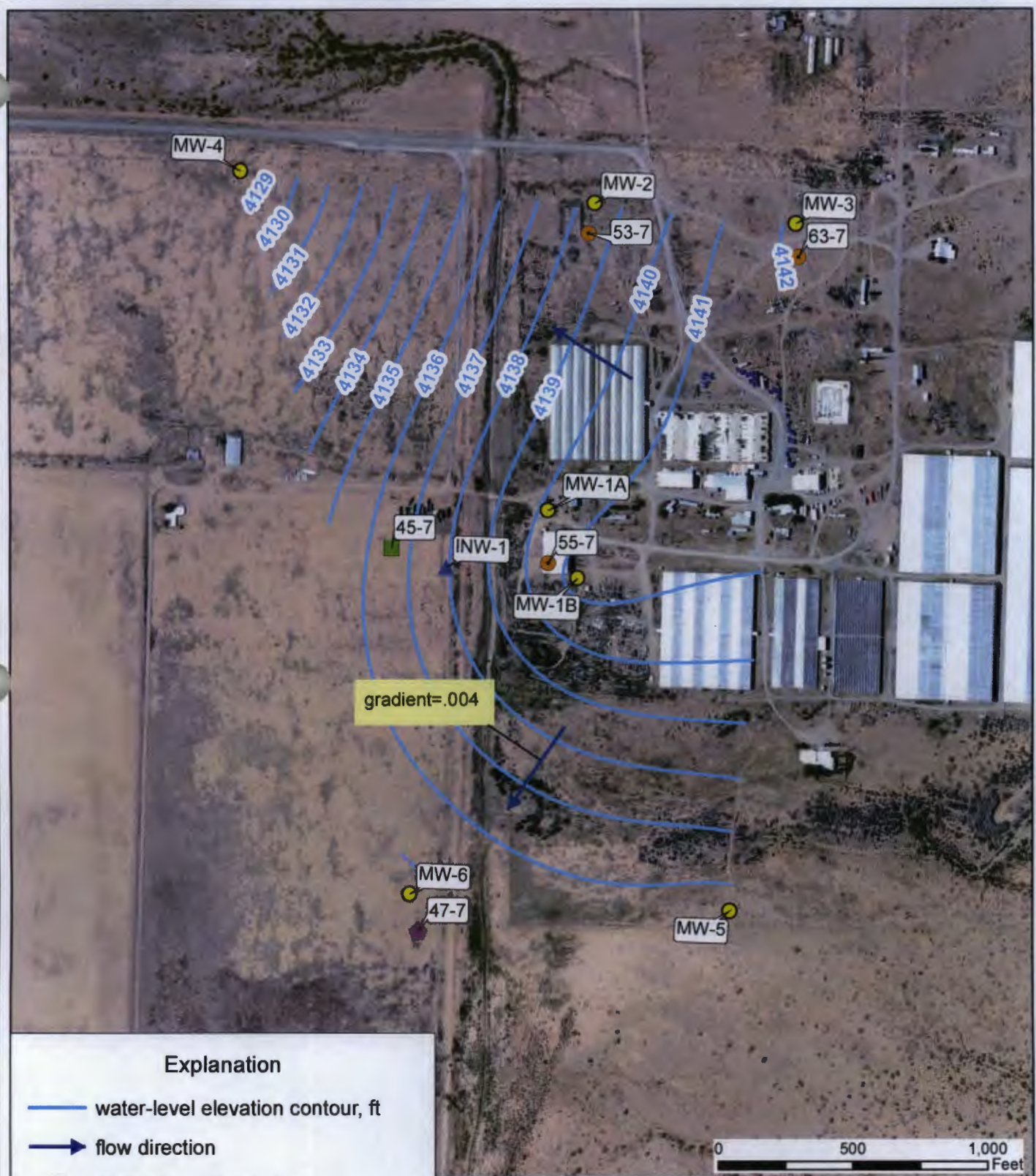
Figure 7. Water-level elevation levels shown in shallow monitoring wells (MW- wells) for February 22, 2014, Cyrq Energy Lightning Dock Geothermal project. Contour values in feet.
