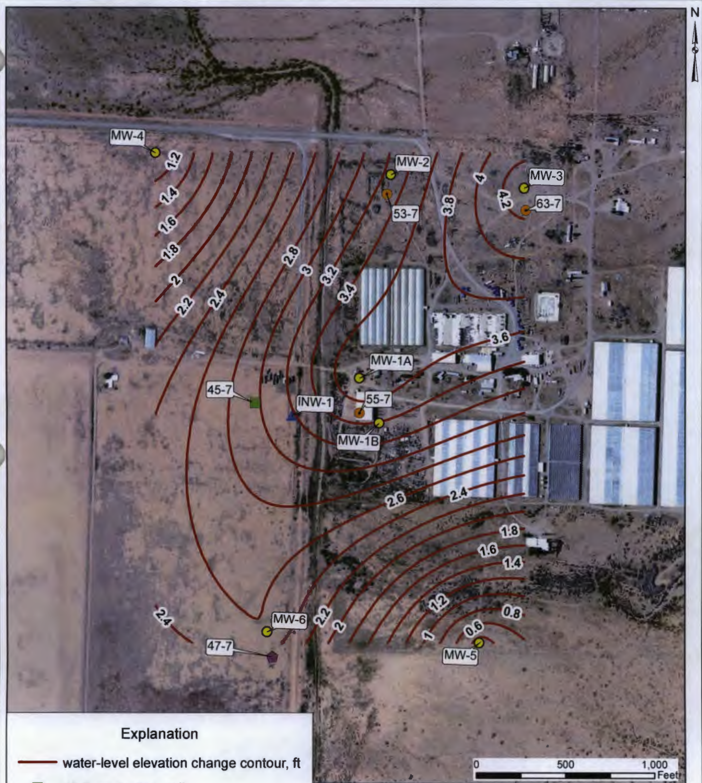
Figure 13. Water-level elevation change in shallow monitoring wells (MW- wells) between December 09, 10, and 11, 2013 (prior to beginning of geothermal operations) and February 22, 2014, Cyrq Energy Lightning Dock Geothermal project. Contour values in feet. Positive value indicates water-level rise.
