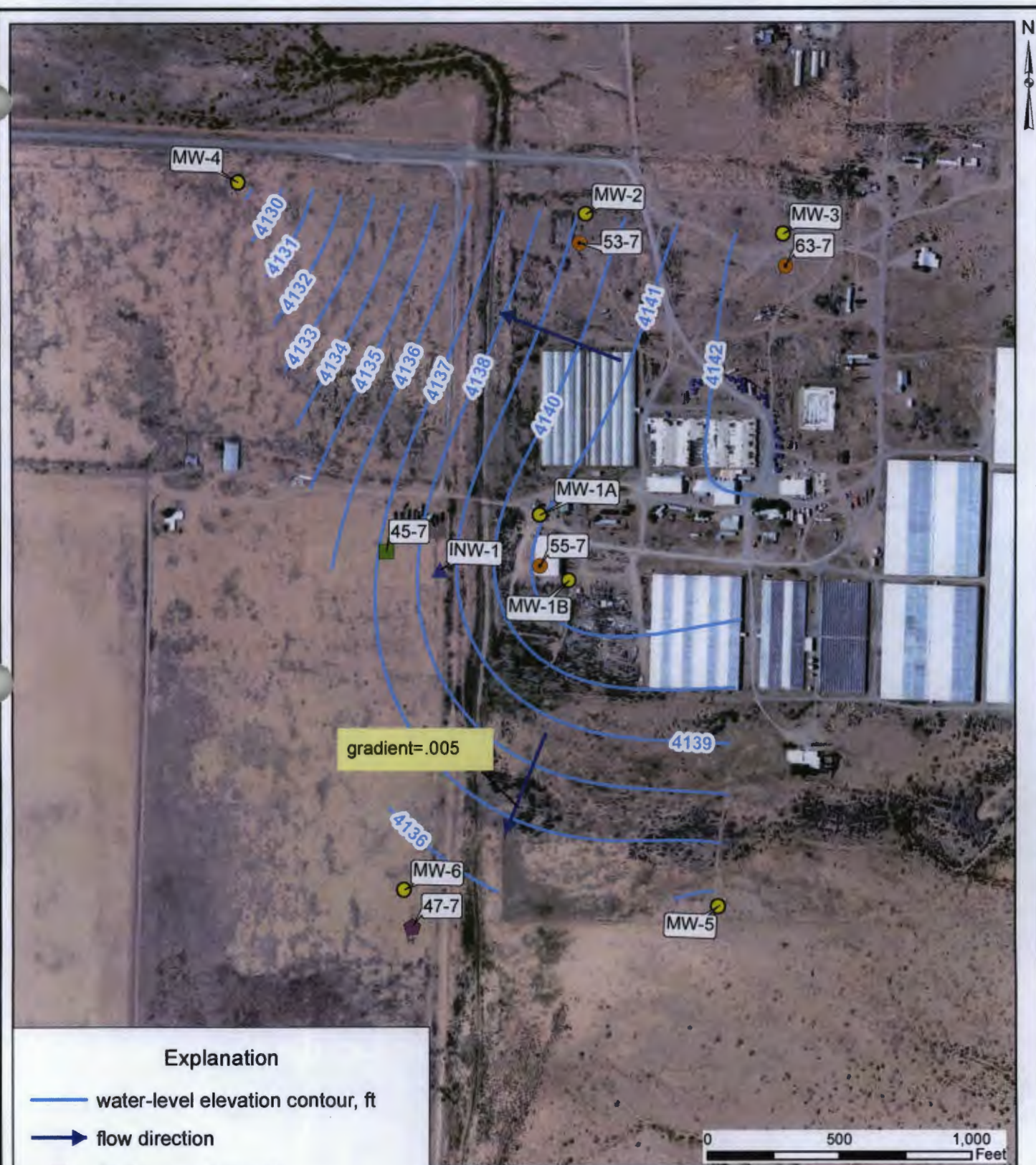
Figure 9. Water-level elevation levels shown in shallow monitoring wells (MW- wells) for April 17, 2014, Cyrq Energy Lightning Dock Geothermal project. Contour values in feet.
