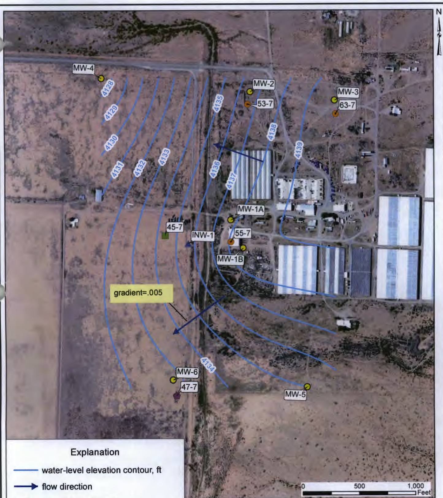
Figure 3. Water-level elevation levels shown in shallow monitoring wells (MW- wells) for December 09, 10, and 11, 2013, Cyrq Energy Lightning Dock Geothermal project. Contour values in feet.
