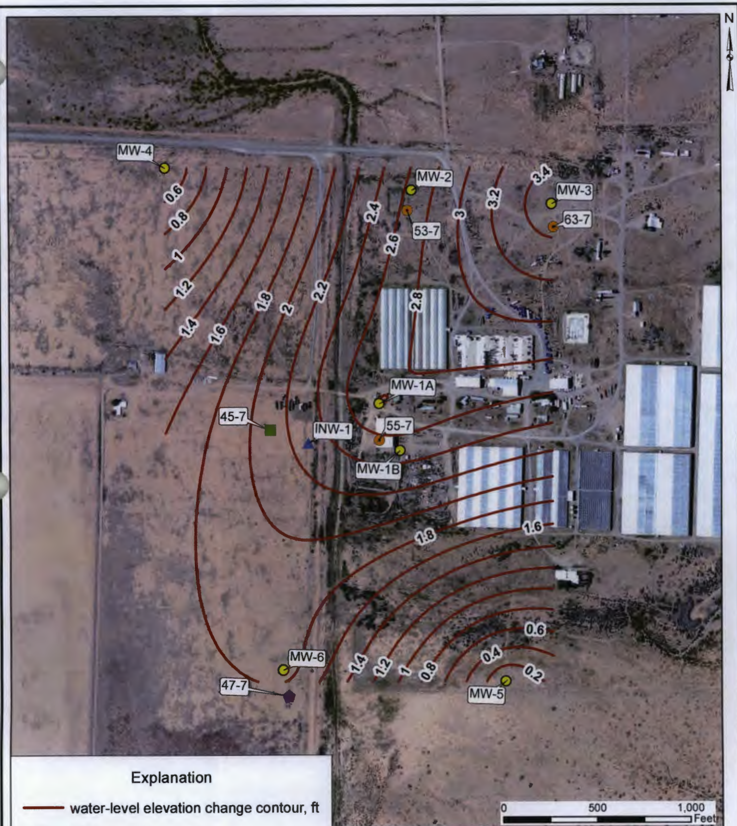
Figure 12. Water-level elevation change in shallow monitoring wells (MW- wells) between December 09, 10, and 11, 2013 (prior to beginning of geothermal operations) and January 27, 2014, Cyrrq Energy Lightning Dock Geothermal project. Contour values in feet. Positive value indicates water-level rise.
