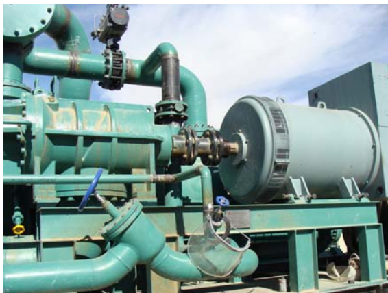
Turbine Screw Turns Electric Generator on Expander Unit
