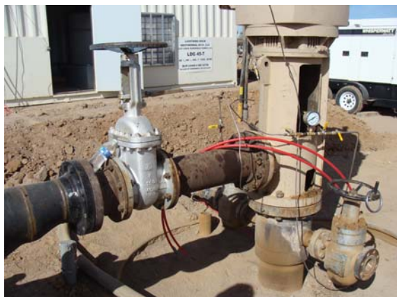
Production Well LDG 45-7 Flexible Poly Pipe connection to Injection Well LDG 53-7
