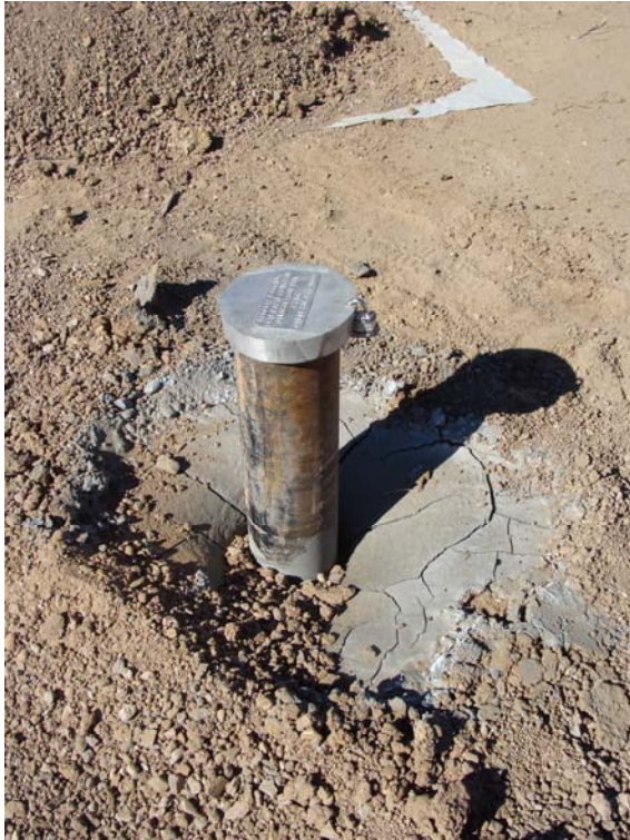
Monitor Well No. 3 (MW-3) Near Injection Well LDG 63-7 with Surface Depression Surrounding Well
