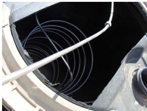
LDG 45-7 ASTM Barrel Bath with Internal Coil Sample Tubing
