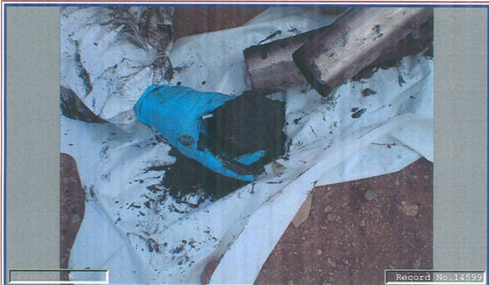
AL1-1 black silty sludge characteristic of the lower portion of most HP samples.
