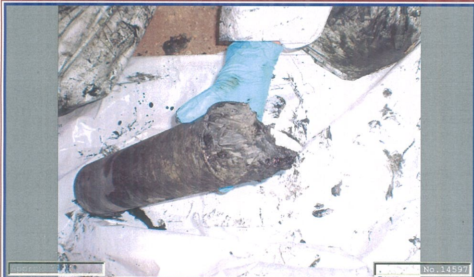
AL1-1 sample in auger core displaying grey clay characteristic of the bottom of both lagoons.
