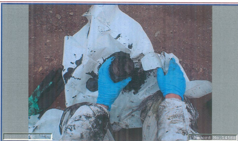
Hardpack sample from AL2-4, characteristic of the hardpack of Aeration Lagoons 1 and 2.
