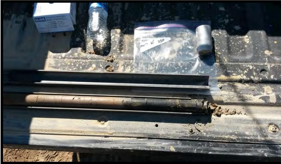
Photo 5: MW-3 is located closest to the location of the release, pictured is the split spoon sample driven from 10 to 12 feet. The black interval is between 11 and 12 feet bgs and had a noticeable hydrocarbon odor.
