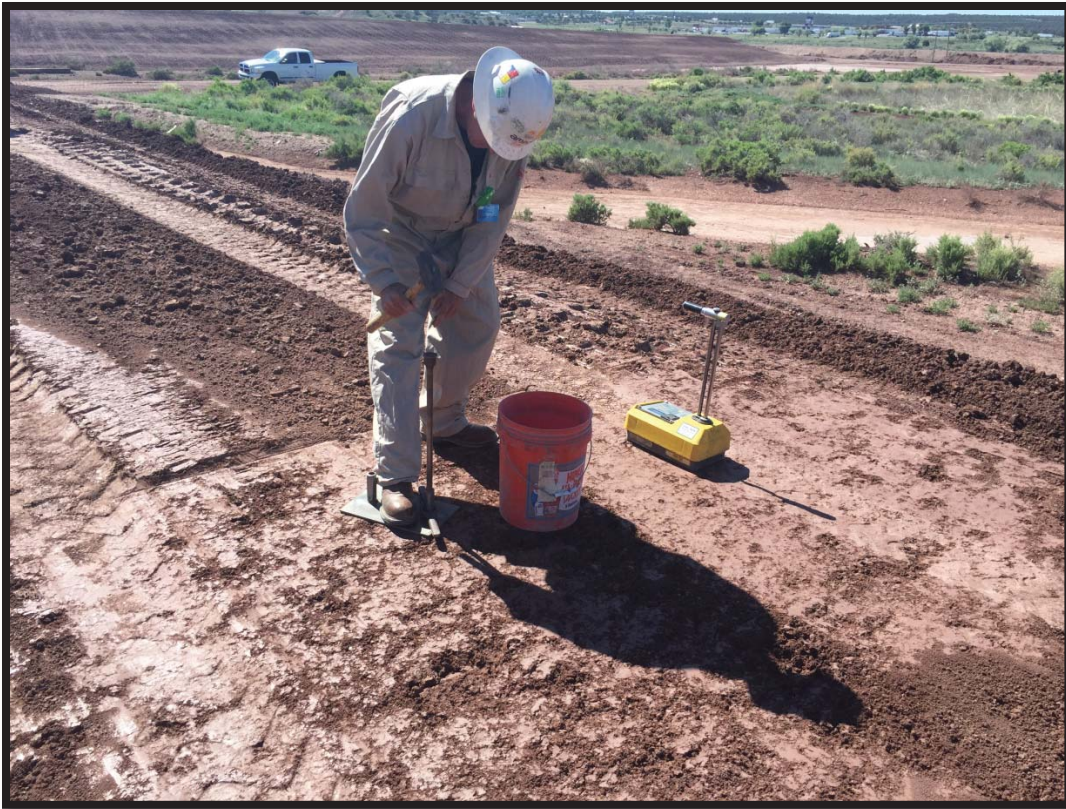
Photo #13: Density Testing Pond 7/8 with repaired Pond 6 in the background
