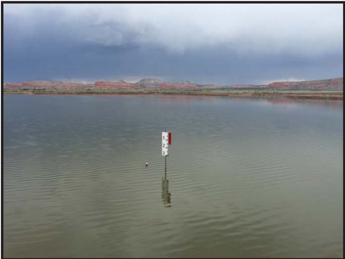
Photo #2: Staff Gauge in Pond 11 - Looking North
