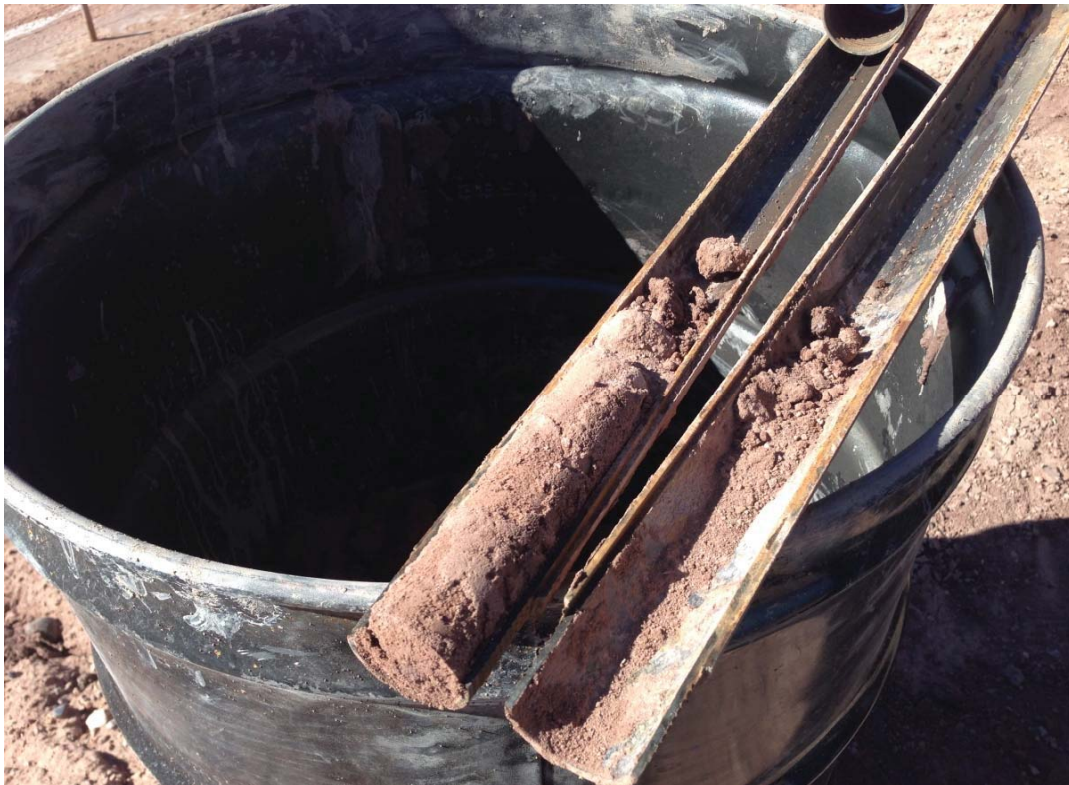
Bottom of Split Spoon Sample from 0 to 2 Feet Deep
