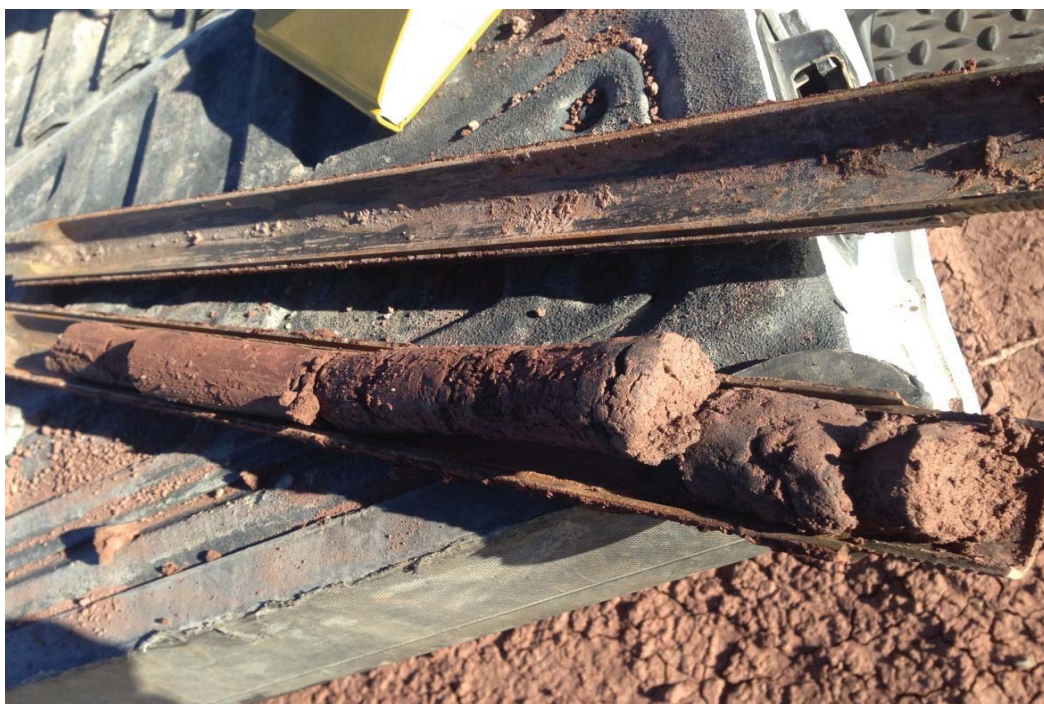
Bottom of Split Spoon Sample from 8 to 10 Feet Deep
