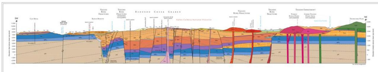
Figure 3. Southwest-northeast cross section through the Valles Caldera. The section transects the Valles and Toledo ring fracture zones, the Redondo Creek Graben, and the Jemez Fault Zone on the southwestern margin of the caldera.<sup>[12]</sup>
