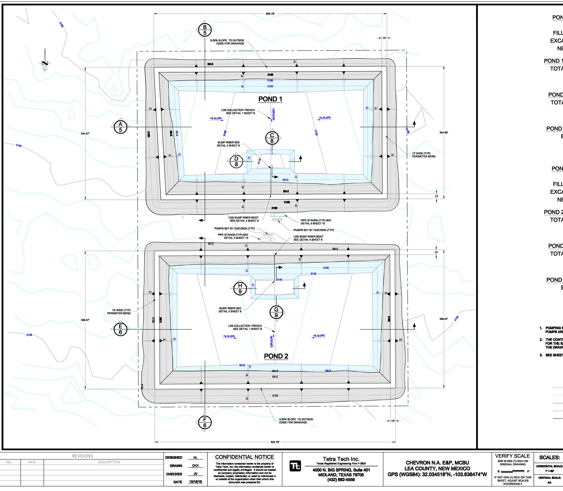
POND 1 EXCAVATION CALCULATIONS TOTAL AREA = 5.98 ACRES FILL VOLUME (1.55x) = 38,247 CU.YDS EXCAVATION VOLUME = 41,443 CU.YDS NET DIFFERENCE = 3,196 CU.YDS.
