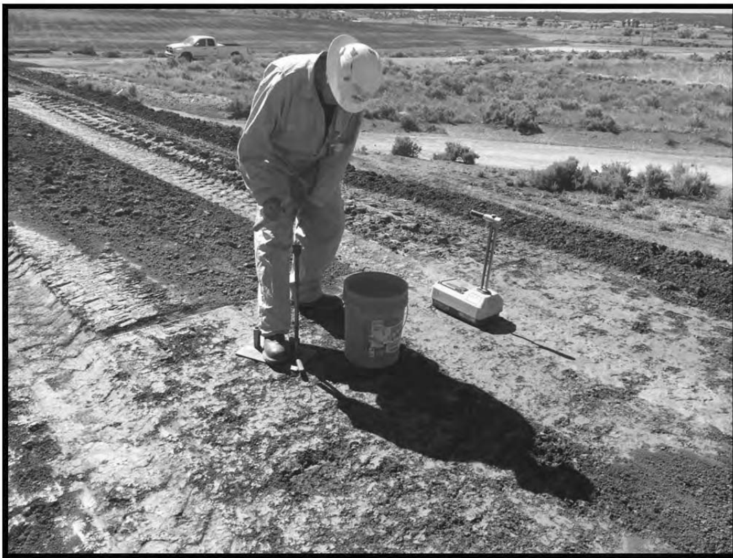
Photo #13: Density Testing Pond 7/8 with repaired Pond 6 in the background
