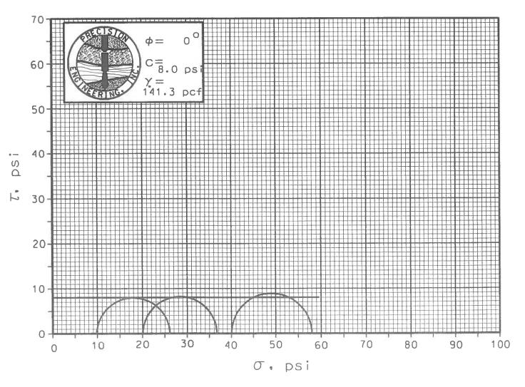
Project: Triza Evaporation agoons Project Number: 00-141 Sample #: 3864 Unit Weight (pcf): 140.0 wet Lateral Pressure =  $\sigma_3$ Max. Deviator Stress =  $\sigma$ Max. Vertical Stress =  $\sigma_1$ () 0 0 σ, Sample  $\sigma_3$ σ ⊥ + \ \ 1 10 12.3 22.3 10+D 2 20 35.9 15.9 €<i 3 40 22.4 62.4  $\overline{\Box}$
