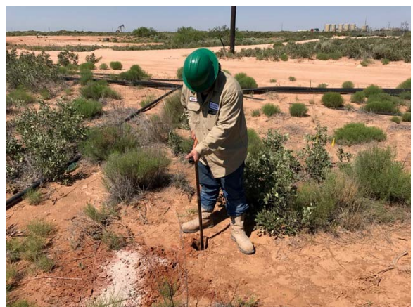
Collecting sample by hand auger
