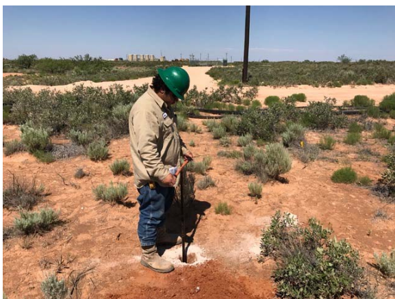
Collecting sample by hand auger
