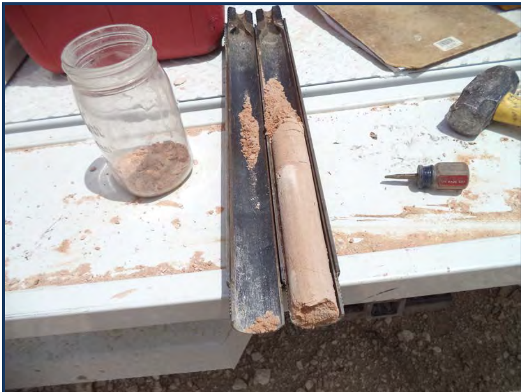
Photograph #4: View of split-spoon soil sample collected from MW-1.
