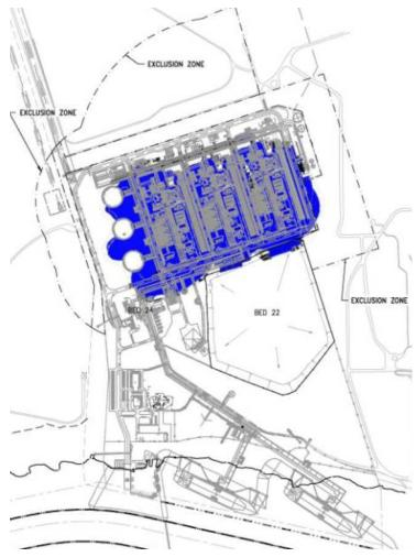
Figure 4.12-3 Vapor Cloud Explosion Overpressure Contours
