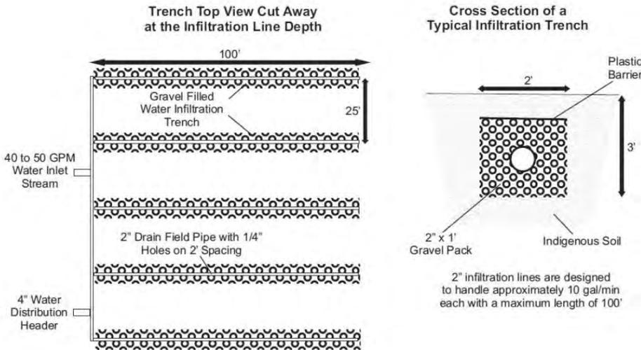
**Description:** Effluent from the treatment system is discharged by gravity to the infiltration gallery. The gallery consists of five horizontally placed perforated pipes that are approximately 1 to 2 feet below ground surface and surrounded by crushed gravel. Each 2-inch diameter infiltration pipe is designed to handle approximately 10 gallons/minute (system total 50 gallons/minute).
