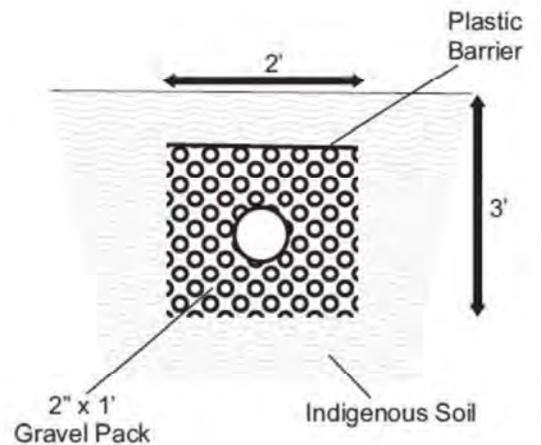
2" infiltration lines are designed to handle approximately 10 gal/min each with a maximum length of 100'
