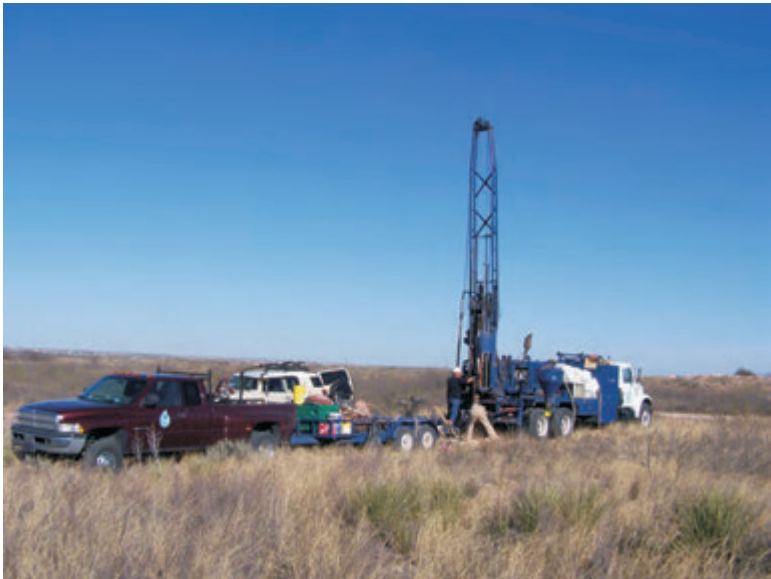
Photograph 9. Rodgers set up on MP-2 with CME-75 combination HSA and air rotary drill rig and related equipment.
