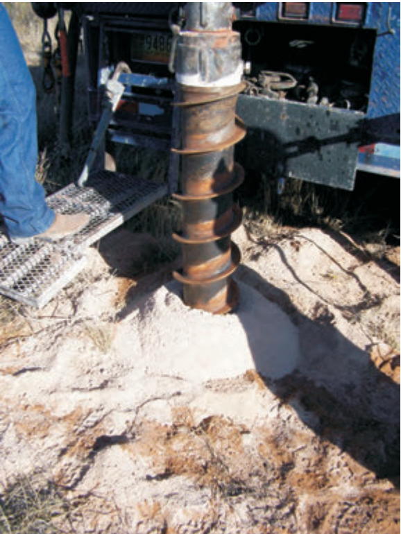
Photograph 10. HSA drilling caliche in boring MP-2.
