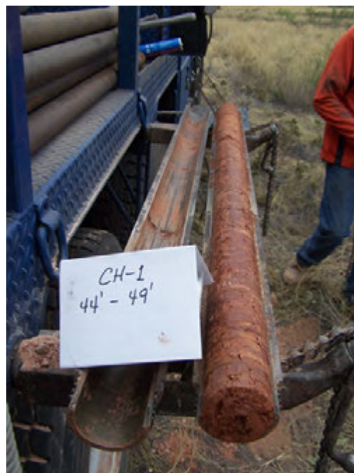
Photograph 4. Core sample of CH-1 at top of Chinle.
