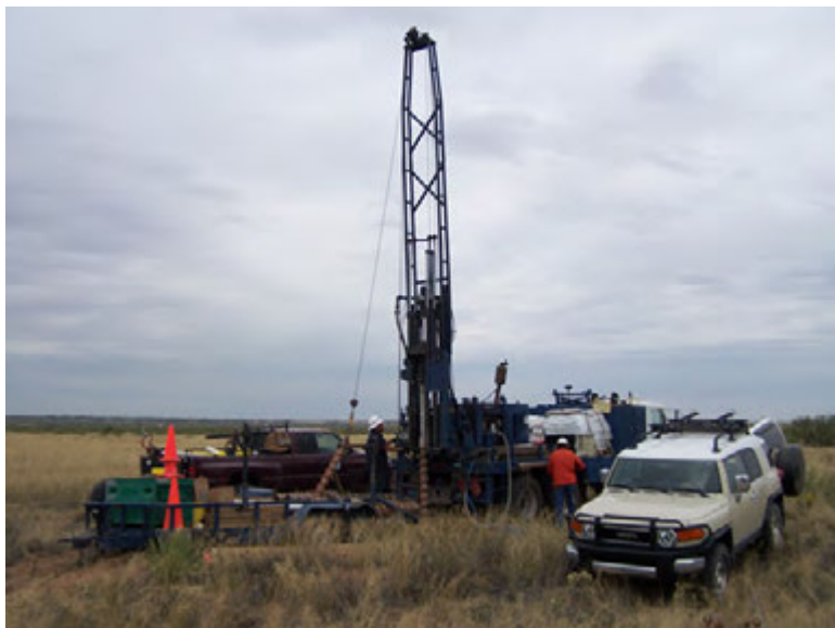
Photograph 1. Rodgers set up on CH-1 with CME-75 HSA and related equipment.
