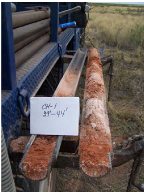
Photograph 3. Core sample of CH-1 at the base of the OAG and top of Chinle.
