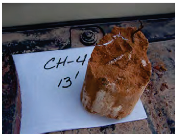
Photograph 24. Root fibers and caliche in sand in upper CH-4.
