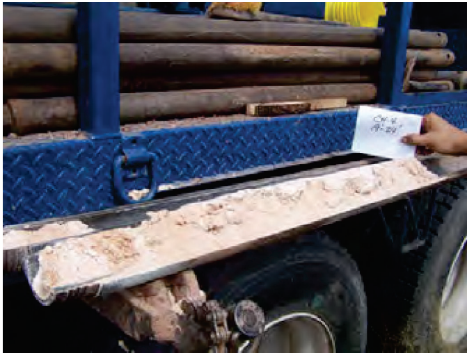
Photograph 25. Core sample of caliche in CH-4.
