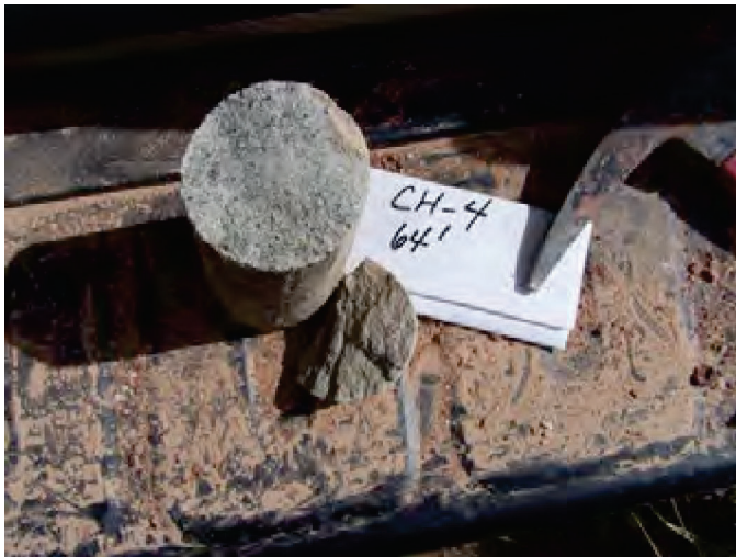
Photograph 27. Core sample of silty sandstone in CH-4.
