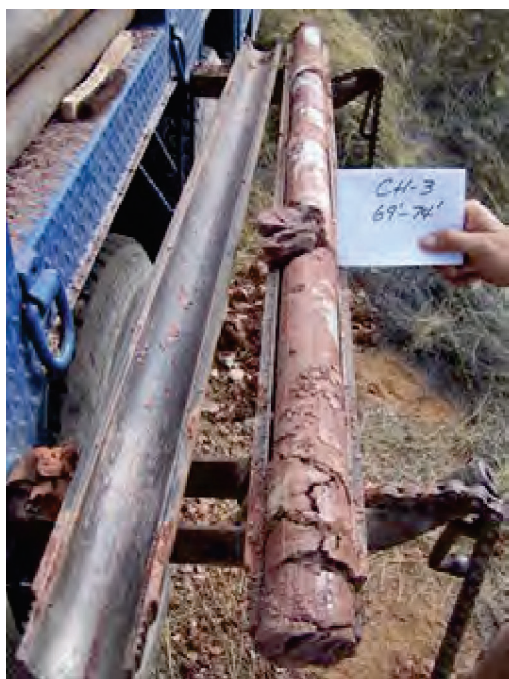
Photograph 21. Core sample of claystone with grey clay inclusions (Chinle) in CH-3.
