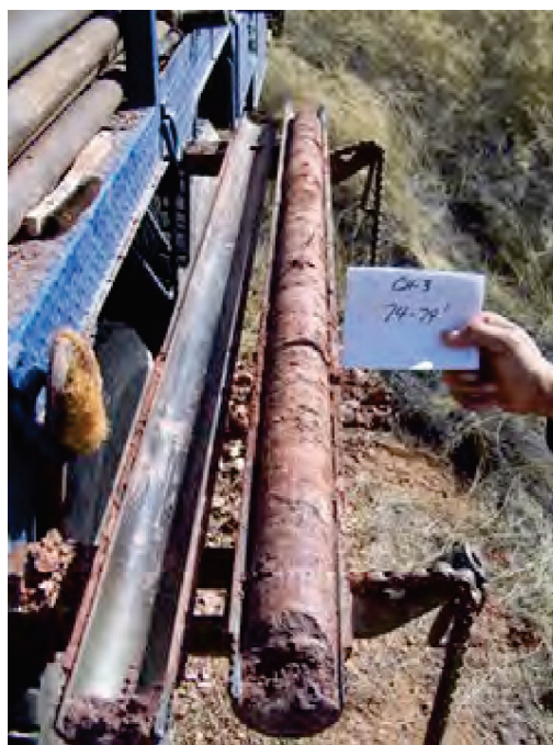
Photograph 22. Core sample of claystone (Chinle) at the base of CH-3.
