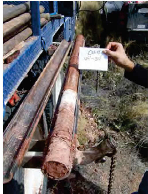
Photograph 26. Core sample claystone (Chinle) in CH-4.
