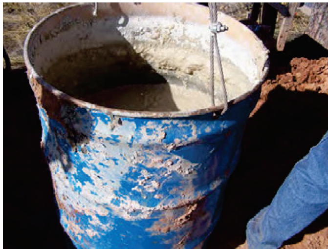
Photograph 35. Typical bentonite-cement grout for plugging boreholes.
