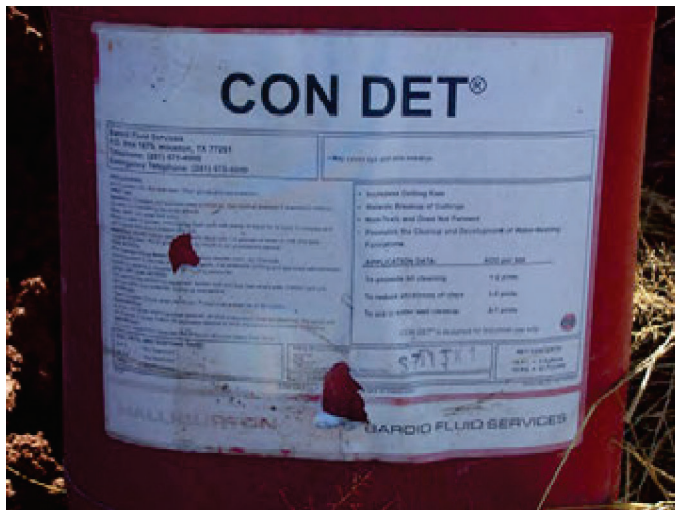
Photograph 33. Con-Det drilling additive for drilling clays.
