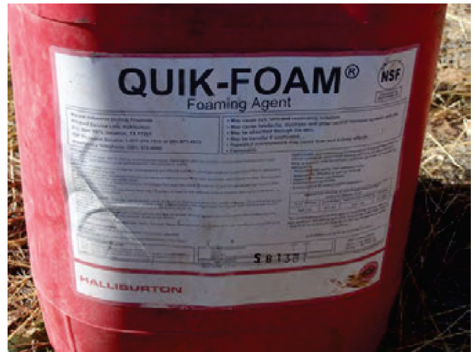
Photograph 34. Quick-Foam drilling additive to retrieve drill cuttings.
