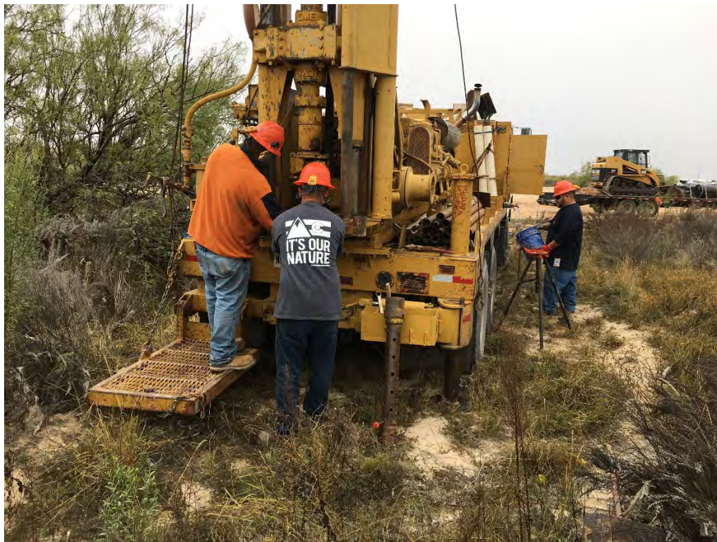
Photo 9.—Hollow stem auger drill equipment and crew
