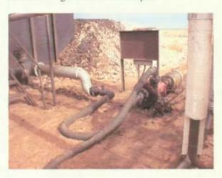
Photo 39 May 31, 2000 Leaking pump/hoses no catchment.
