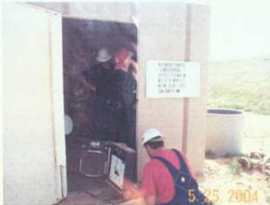
Well House- rigging up pressure chart recording for MIT test. See well file for results and chart.
