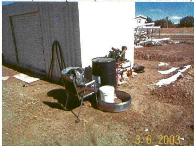
Photo 1. Storage shed area. Barrel and bucket are not on secondary impermeable containment. Landfarm berm is continued around the shed.
