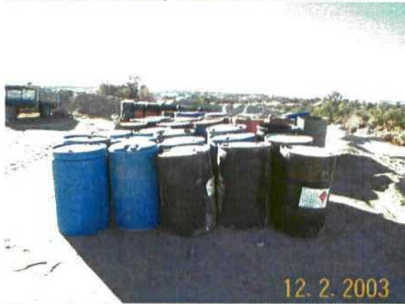
Photo 13. . Drums are stored along a drainage. Drum storage area is not bermed and is not impermeable. Drums are not clearly labeled.
