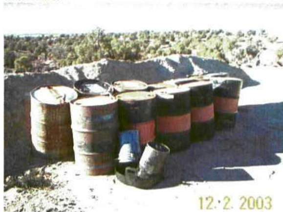
Photo 15. Drums are stored along a drainage. Drums are not labeled and they are not on an impermeable bermed containment.
