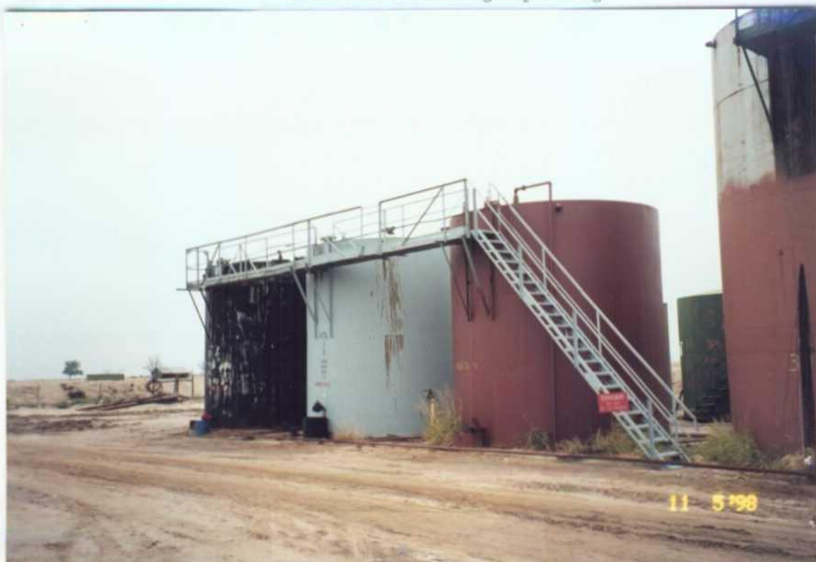
Photo Number: 5 Photographer: T. Reeves, SAIC Location: Gandy Corporation Subject: Tanks used for storage of tank bottoms. City/County: Lea County State: NM Date: 11/05/98 Time: pm Weather: cloudy, cold
