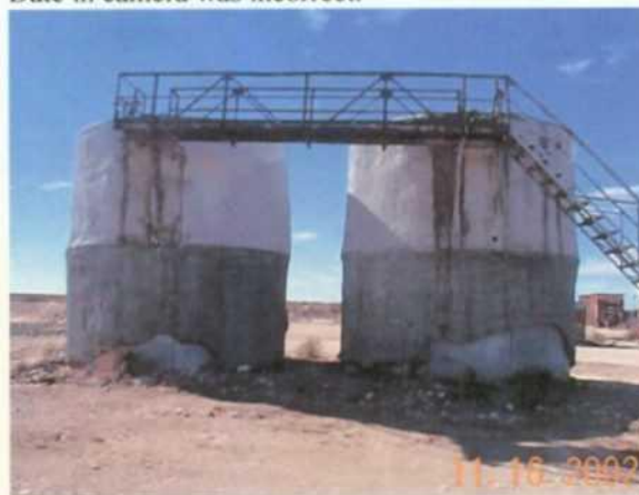
Photo 22. Insulated tanks containing junk oil from the initial pit remediation and recycling project.
