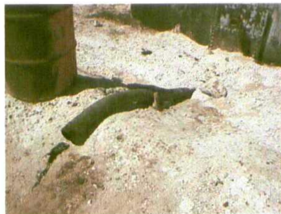
Photo 18 04-13-00 Hose draining directly to ground.
