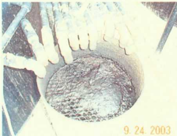
Photo 8 Barrel is over \frac{2}{3} rd full and needs to be emptied to prevent a potential overflow.
