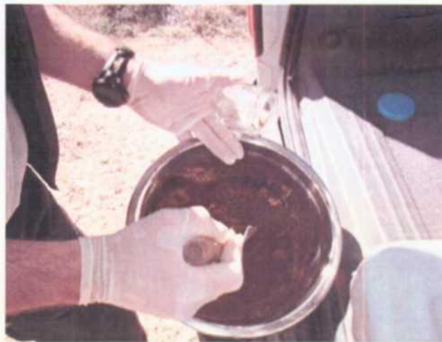
Mixing composite sample of Cell 23
