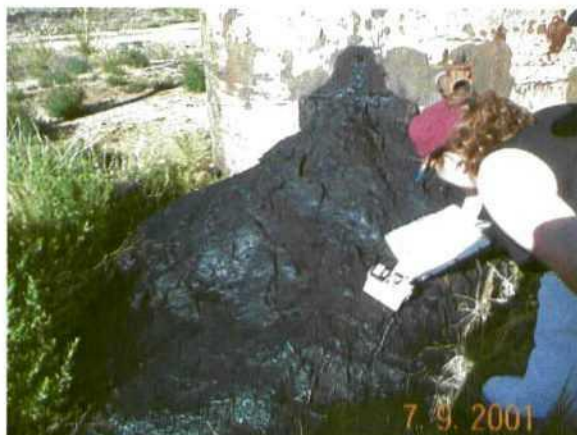
Photo 1: Tank #1 (north tank) with hydrocarbon material that has leaked out of a hole.
