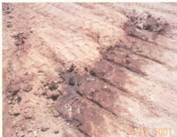
Contaminated soil beneath tanks
