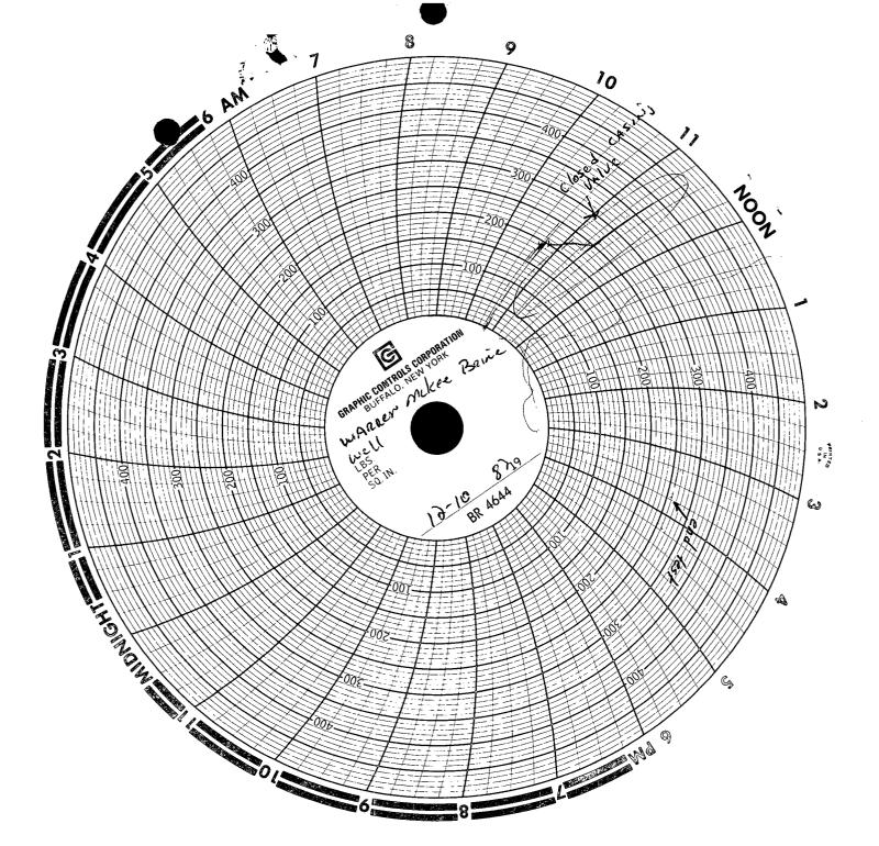
AGENCY LETTERHEAD Location WARREN Make Date 12-10-87 \_\_\_\_\_To\_\_ Location BRINE Well DP-318 From Subject BRINE well Pressure test Pressured casing tubing and cavity to 260 PSI GAULE at 11:25 AM 12-10-87. Pressure reading time 11:25 260 11:35 260 11:45 260 11:55 260 12105 260 12:15 760 12:25 260 · 9:33 260 3:25 260 test completed at 3:25 pm 12-10-87 Jearl Petre
