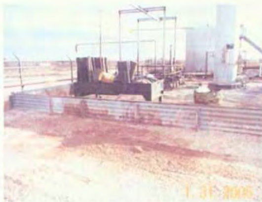
Oil Treater-SE part of plant-oily stains in area.
