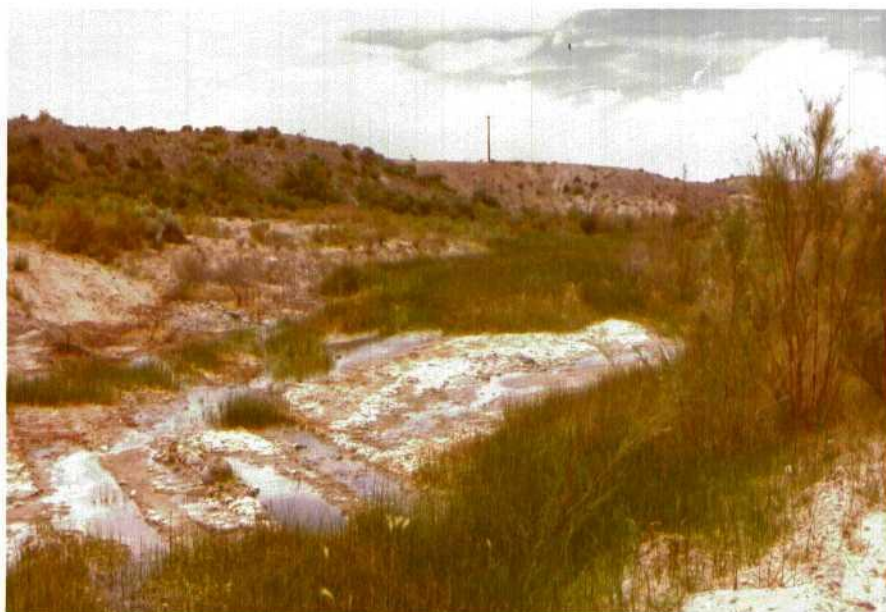
Figure 12. Photograph showing gravel pit excavated in the cobble which has exposed the underlying Nacimiento Formation. At the contact, oily water is seeping from the cobble bed. The occurrence is on the western side of section 27, T. 29 N., R. 11. W. The area is upgrate on the Nacimiento subcrop from the Plateau Refinery and the oily water is not derived from refinery operations.
