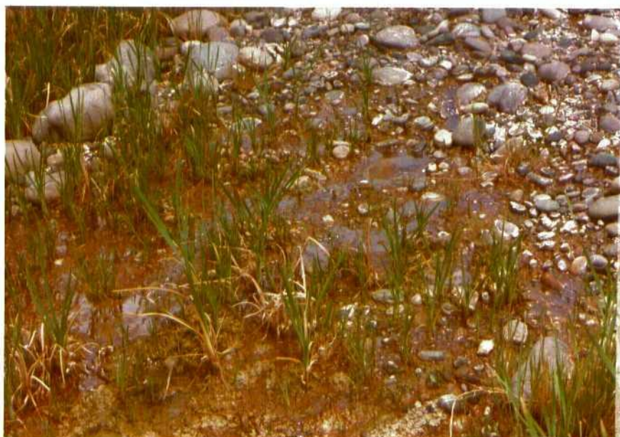
Figure 14. Close up of the contact between the Pleistocene cobble and the Nacimientto Formation shown in figures 13 and 14. The greenish Nacimientto Formation is in the lower part of the picture. View shows the seep of water at the contact.
