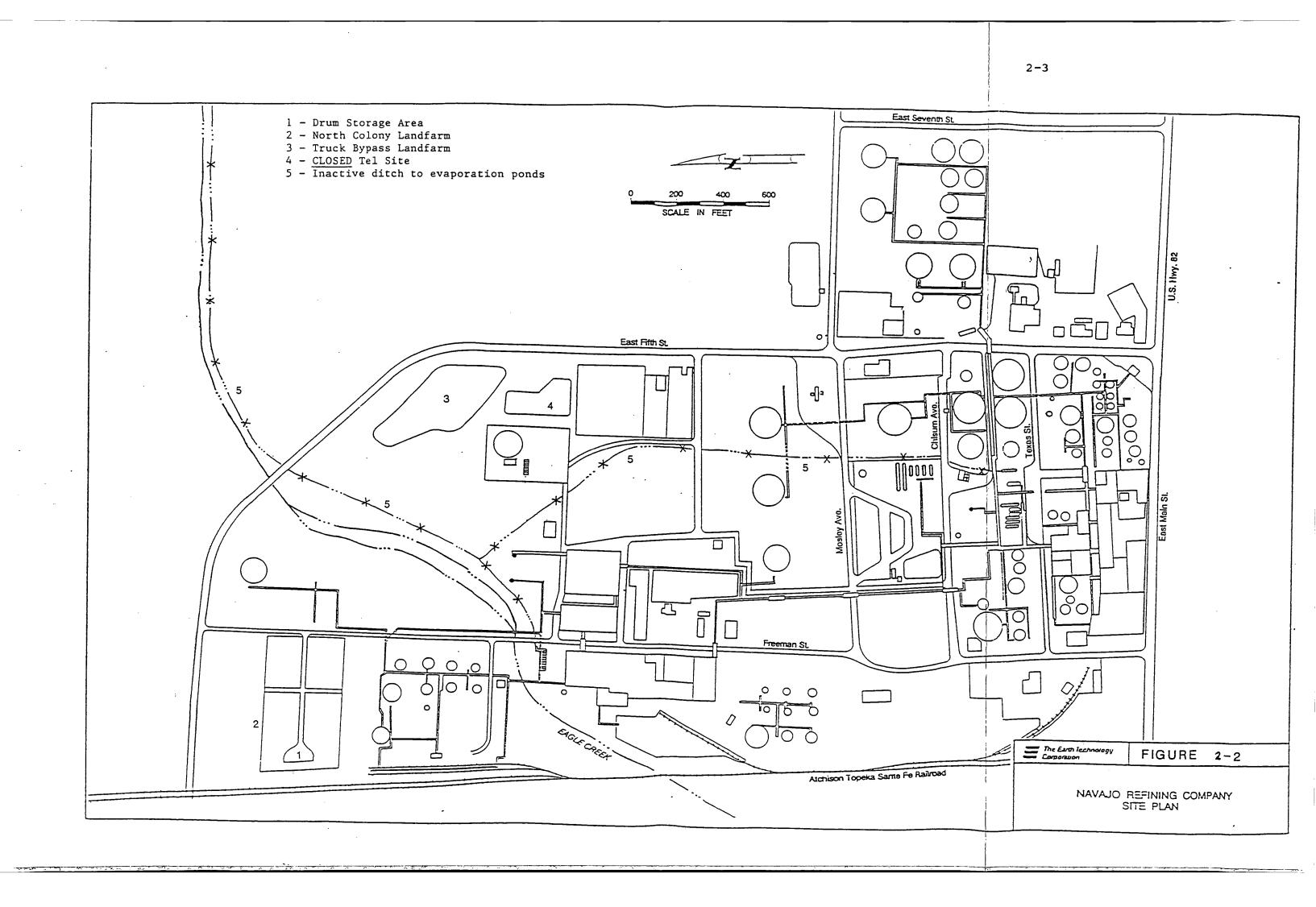
Colony Landfarm. The wastewater management system presently employed by Navajo consists of a wastewater treatment plant and a system of evaporation ponds.
