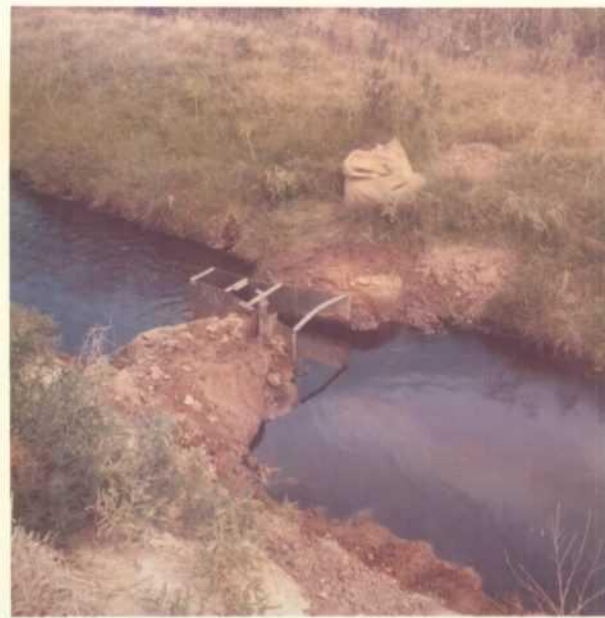
Six-inch Parshall Flume Looking Downstream (Location B)
