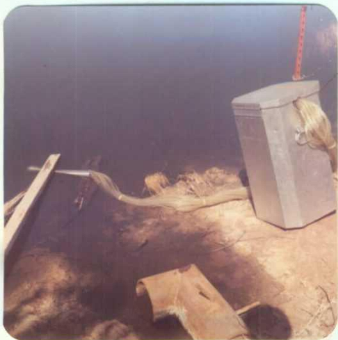
Composite Sampler set up on Effluent From Number Two Lagoon. (Location M) Looking Southwest
