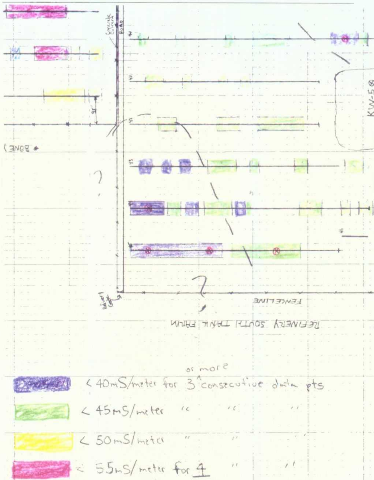
Figure 2. Example of color and visual evaluation of EM Survey numerical data
