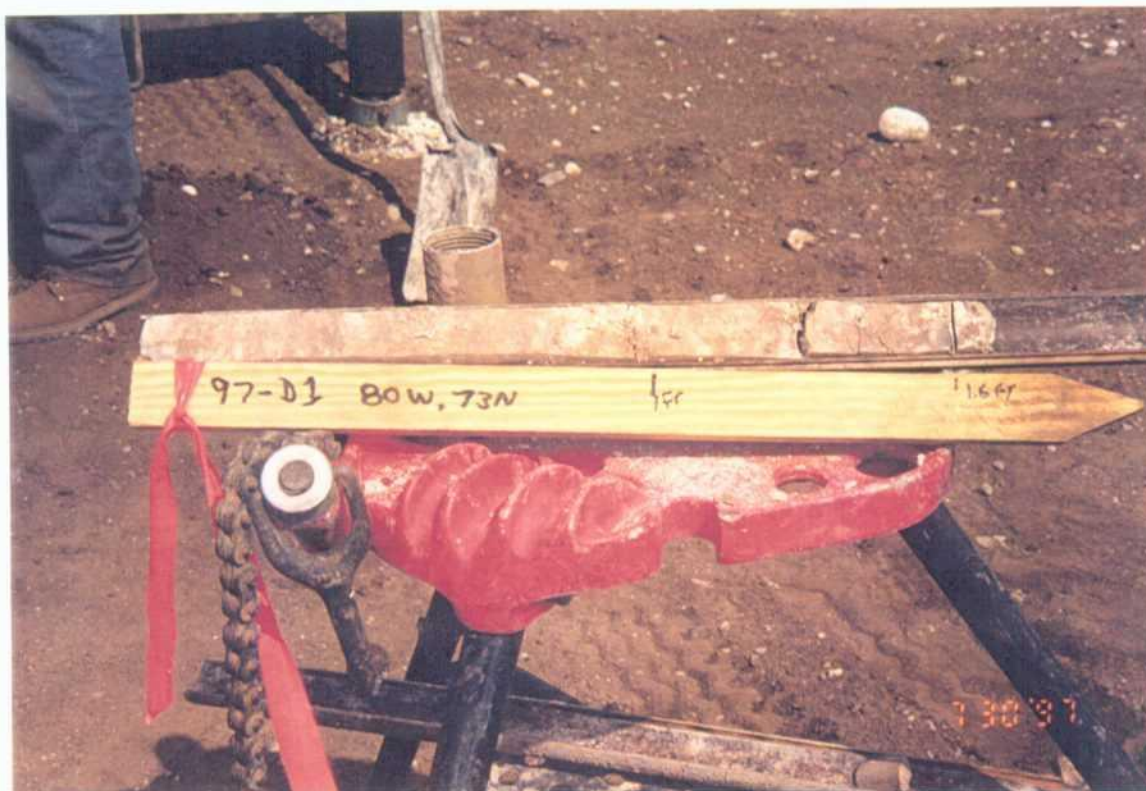
Photograph A-39: Boring 97-D1, Splitspoon; left 17 ft; right, 15 ft.
