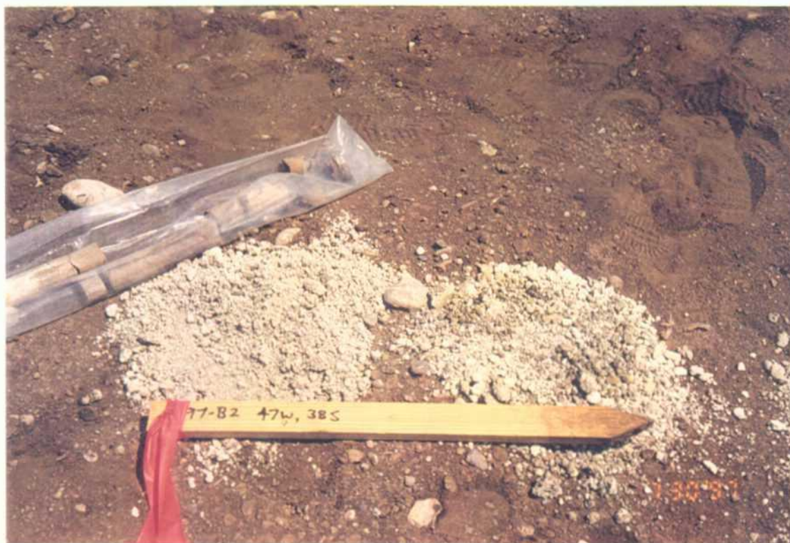
Photograph A-23: Boring 97-B2, left, 13-15 ft.; right, 10-13 ft.
