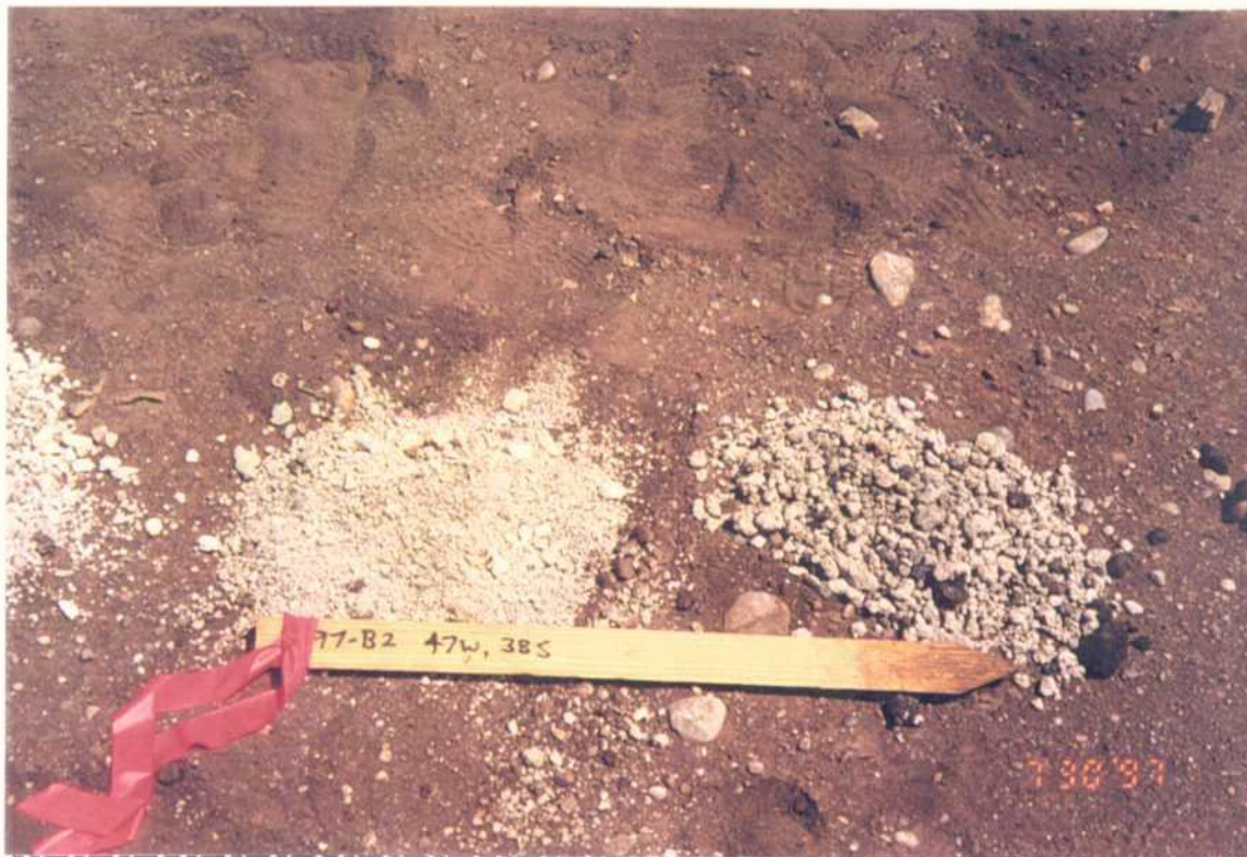
Photograph A-22: Boring 97-B2, left, 8-10 ft.; right, 5-8 ft.
