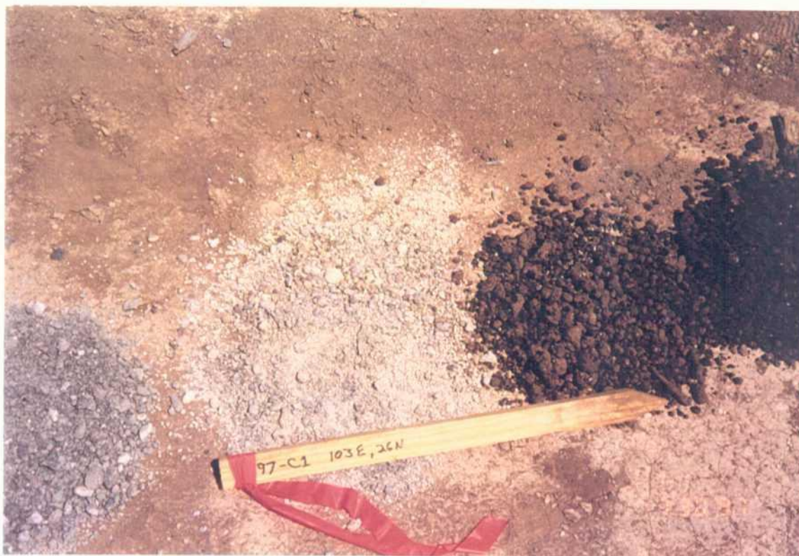
Photograph A-30: Boring 97-C1, far left, 10-13 ft.; left, 8-10 ft.; right, 5-8 ft.; far right 2-5 ft.
