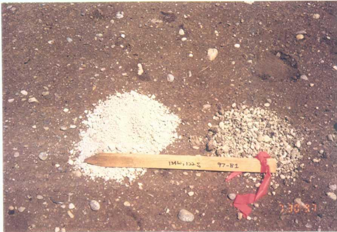
Photograph A-19: Boring 97-B1, left 13-15 ft.; right 10-13 ft.
