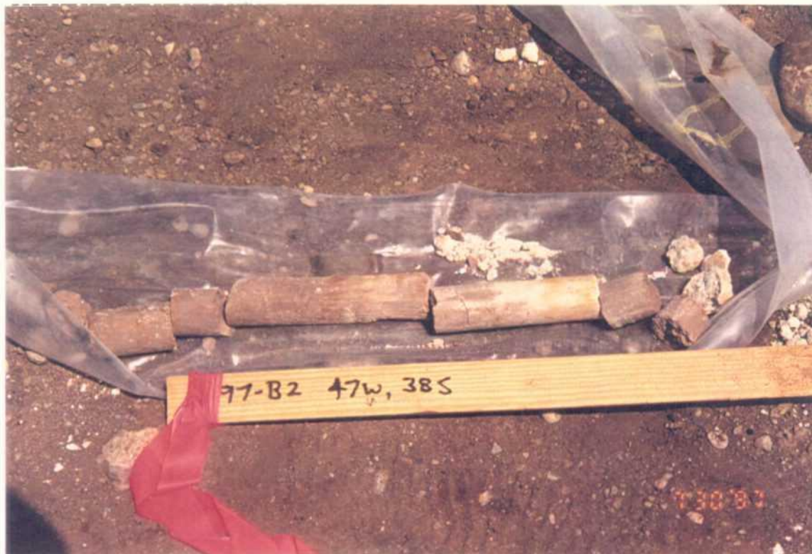
Photograph A-24: Boring 97-B2, Splitspoon, left, 17 ft.; right, 15 ft.
