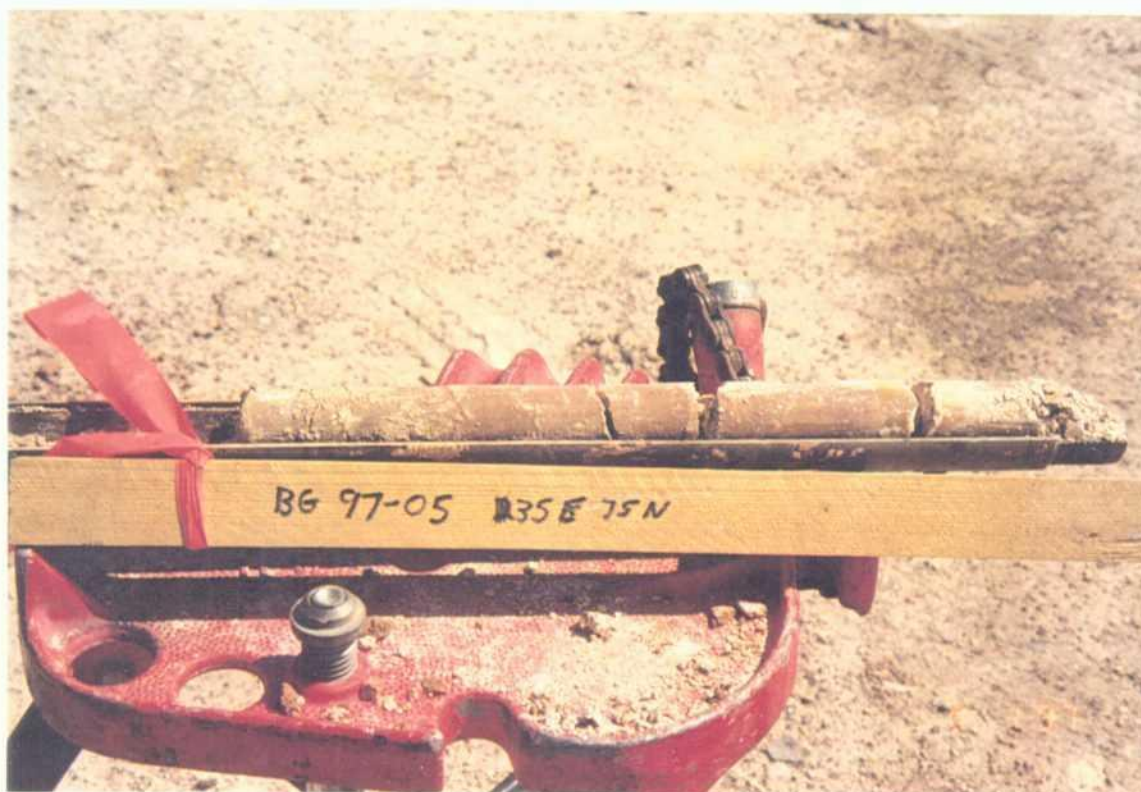
Photograph A-44: Boring BG 97-05, left, 7 ft.; right, 9 ft.
