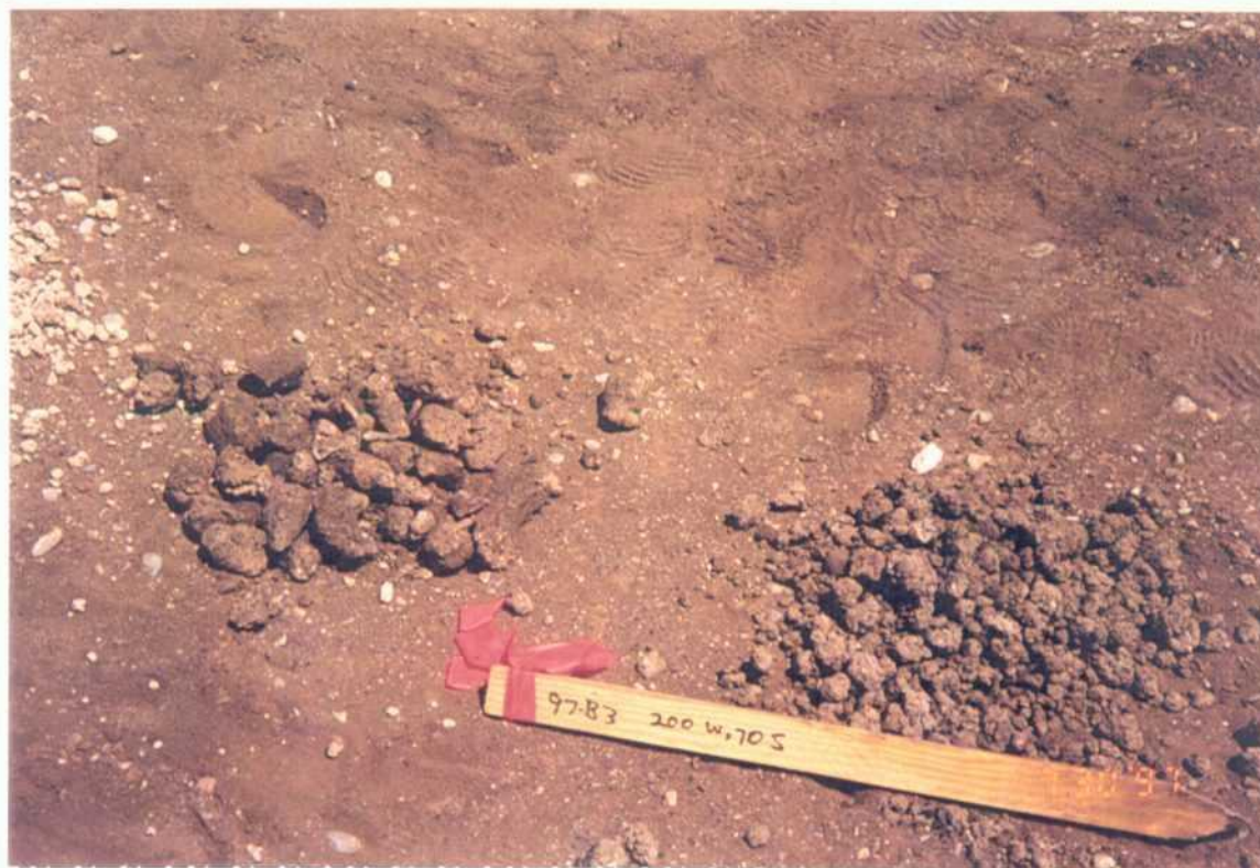
Photograph A-26: Boring 97-B3, left, 8-10 ft.; right, 5-8 ft.
