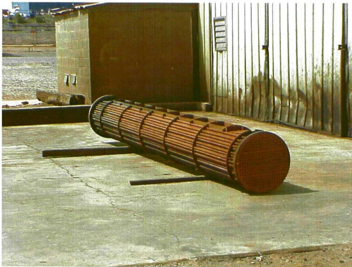
Photo 3 A clean heat exchanger bundle at the <90 day storage unit, facing north
