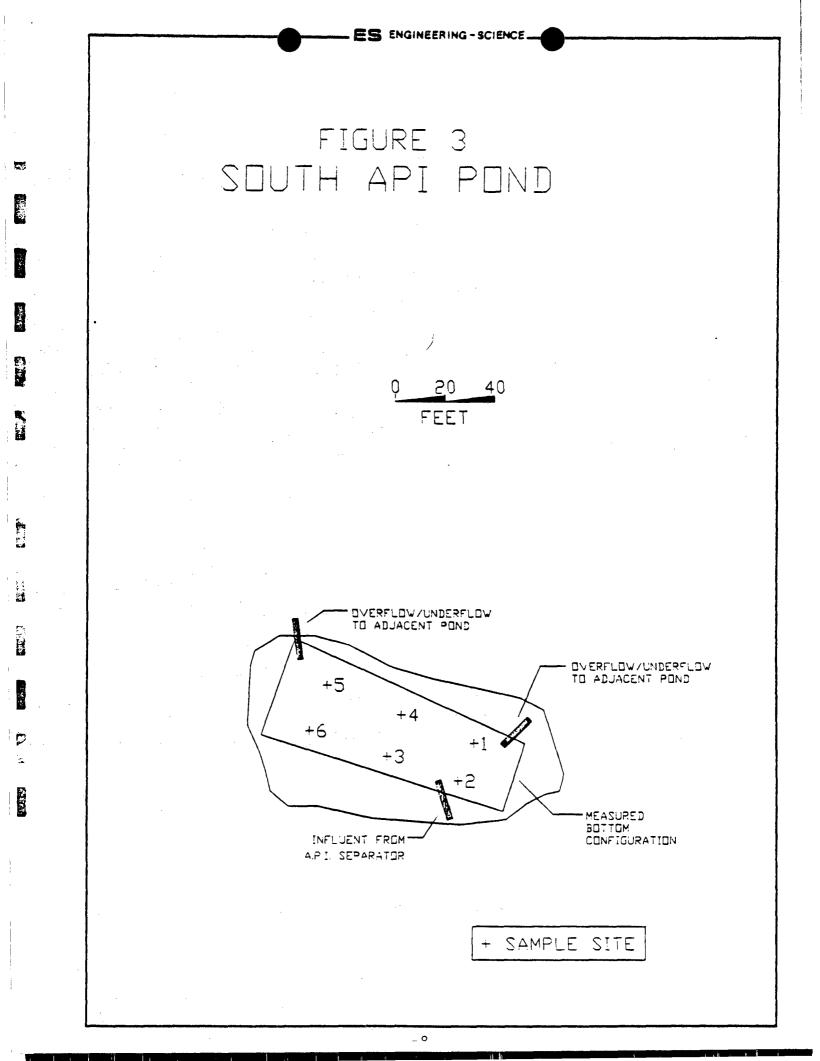
In the south API wastewater pond, a single grab sample collected in the top 6 inches near the influent end of the pond was analyzed for the "Skinner List" of compounds expected to be present in petroleum refinery wastes. This list and the analytical methods being used are presented in Table 1. None of the "Skinner List" constituents were present at detectable concentrations in this sample.
