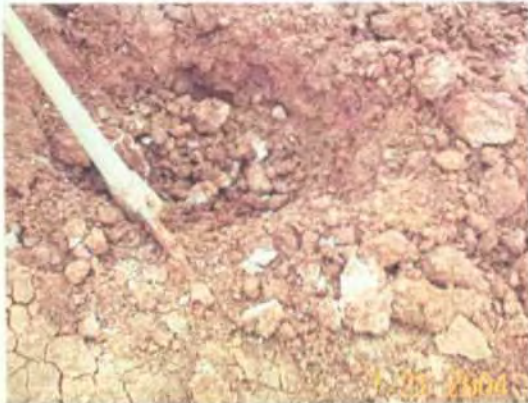
Picture of area where soil sample collected for re-testing by Pettigrew Assoc. Located on north side of pond sidewall approximately half way up. Noted dry clayey soils with some silt, caliche fines and gypsum roses.
