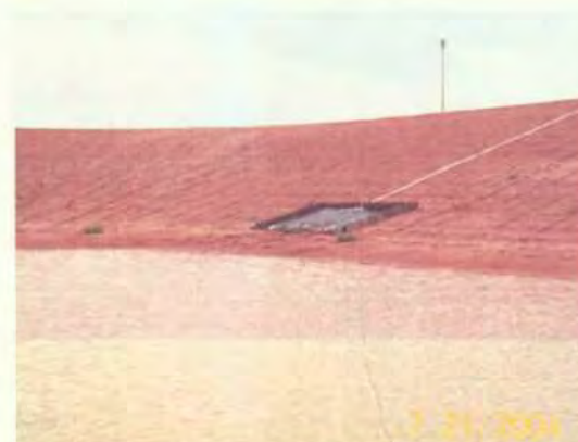
Apron where pond was partially filled for infiltration test. Large recent rain filled the bottom with about one foot of water.
