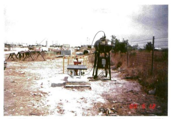
View facing north showing Xitech product recovery system installed at recovery well RW-1.
